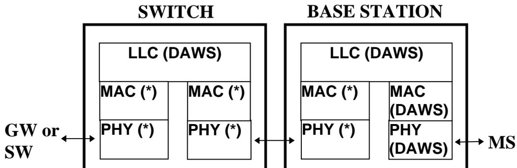
Figure 8: DAWS Switch to Base Station Protocols
