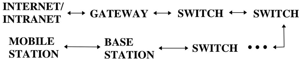
Figure 6: DAWS Maximum Complexity Network Architecture
