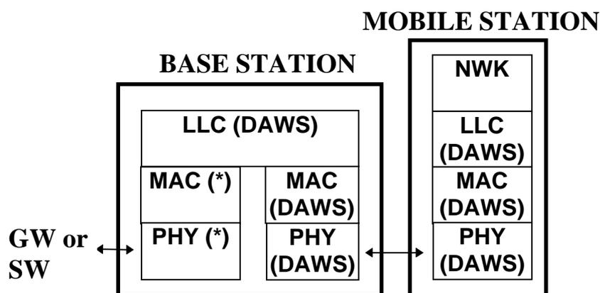
Figure 9: DAWS Base Station to Mobile Station Protocols
