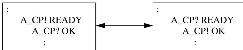
**Figure 6 - Example of a simple handshake**
