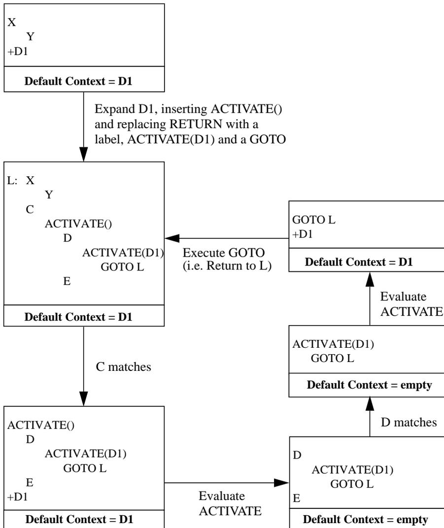
Figure 10 - Possible progression of evaluation of example test case X-Def3
