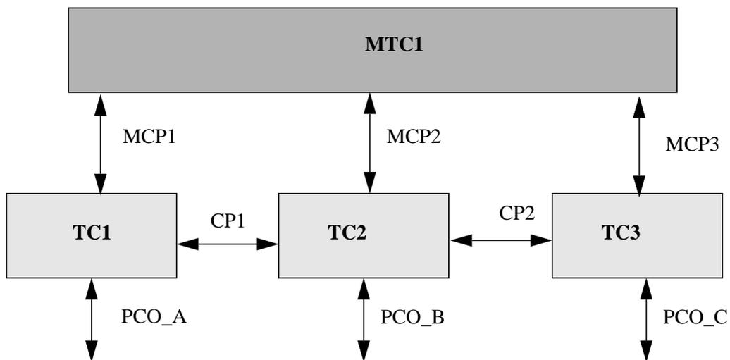
Figure 3 - Example Test Component Configuration CONFIG1
