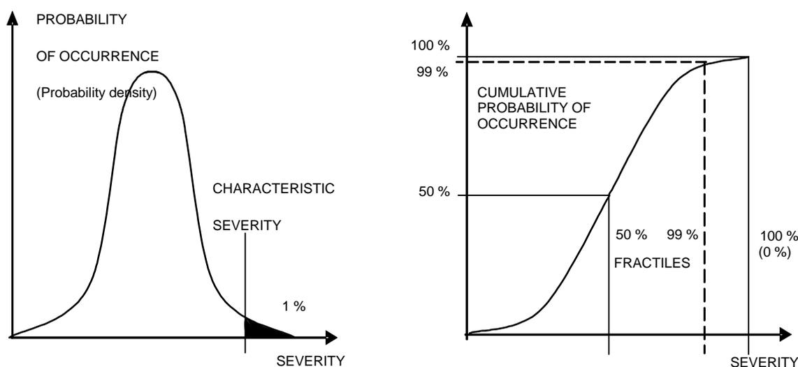
**Figure 4: Schematic example showing the occurrence of the severity of a parameter (e.g. level of aggressive pollutant)**
