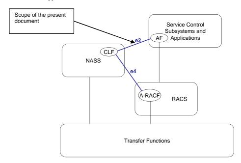
Figure A.1: NASS external interfaces
