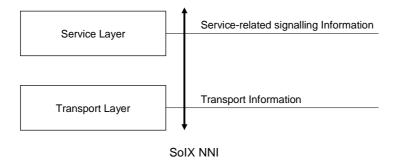
Figure 7a: Solx Interconnection architecture and NNI
