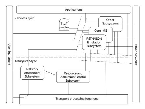
Figure 1: TISPAN NGN overall architecture
