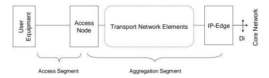
Figure 2a: Access and aggregation segments
