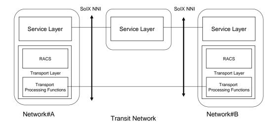
Figure 7i: Indirect Interconnection with service layer intermediary
