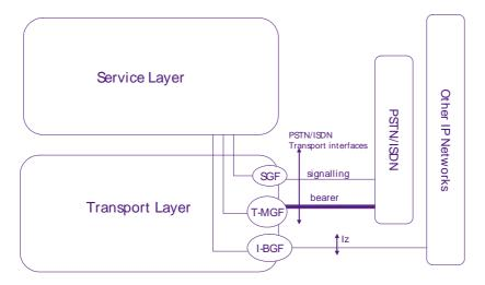
Figure 5: Network interconnection at transfer level
