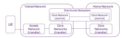
Figure 2: Distributed subsystems
