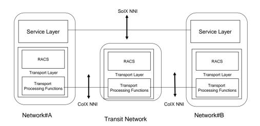
Figure 7j: Indirect Interconnection with transport layer intermediary
