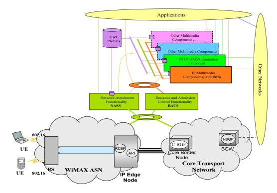
Figure C.1: Example architecture with WiMAX access
