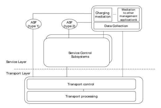
Figure 4a: Charging and Data Collection Functions
