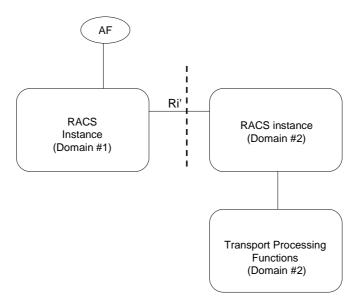
Figure 6a: Network interconnection at the RACS level
