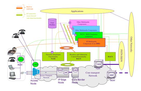
Figure A.1: Example architecture with xDSL access
