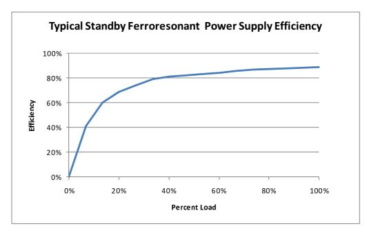
Figure A.1: Typical standby ferroresonant power supply efficiency
