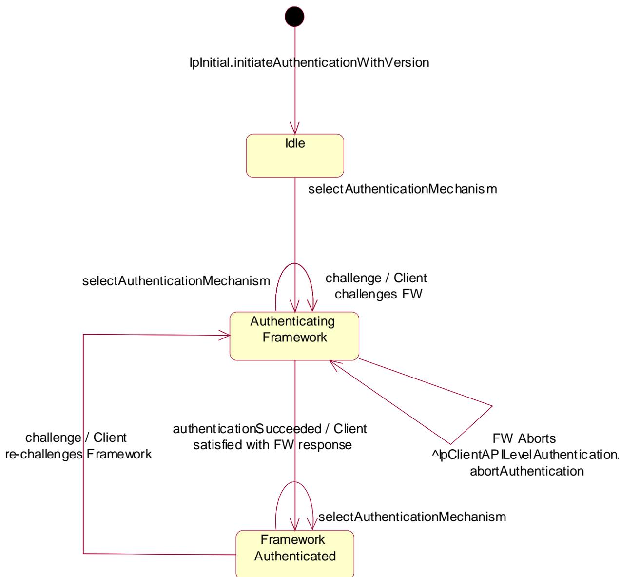
**Figure 3: STD for IpAPILevelAuthentication: Client authenticates Framework using initiateAuthenticationWithVersion() and challenge() method combination**
