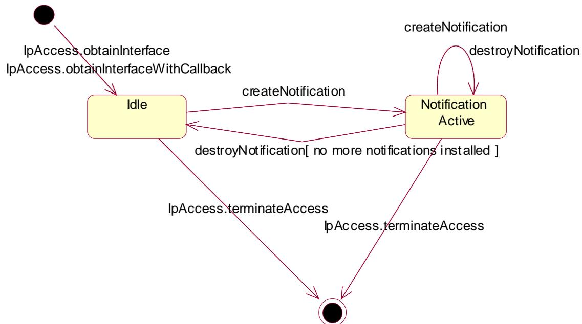
Figure 16: State Transition Diagram for IpEventNotification
