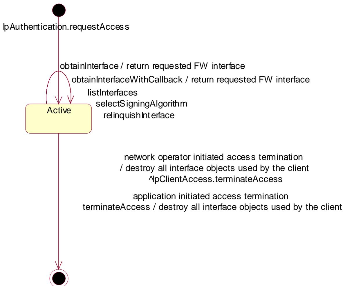
Figure 7: State Transition Diagram for IpAccess
