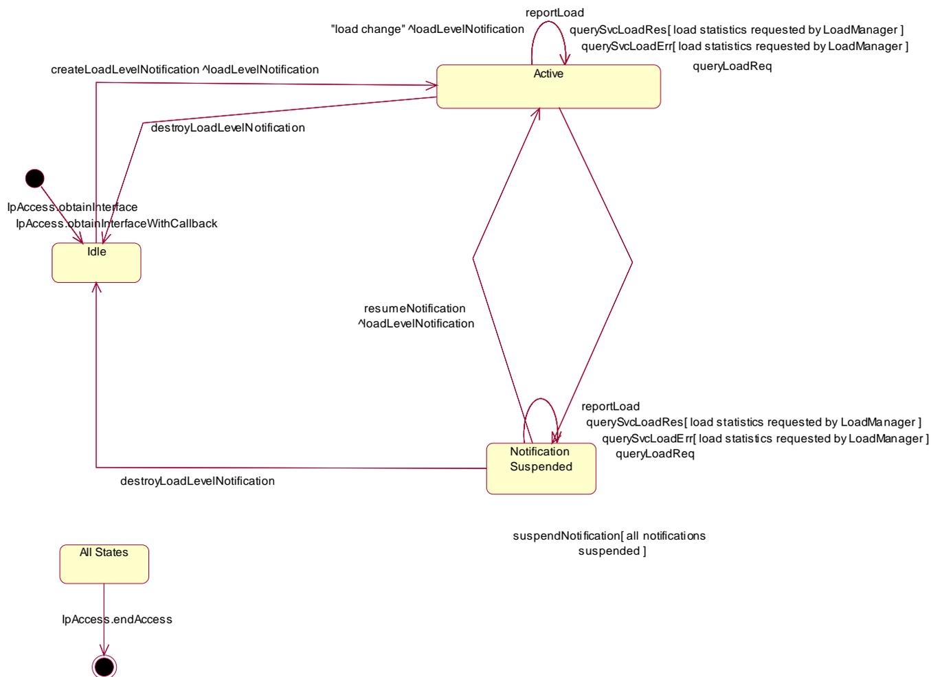
**Figure 14: State Transition Diagram for IpLoadManager**
