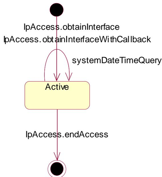
**Figure 16: State Transition Diagram for IpOAM**
