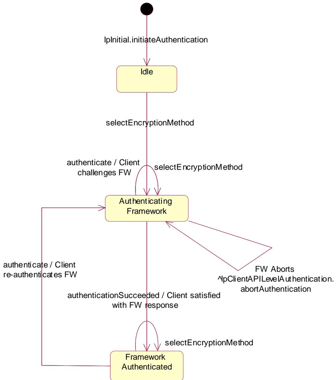
**Figure 3: STD for IpAPILevelAuthentication: Client authenticates Framework using deprecated initiateAuthentication() and authenticate() method combination**
