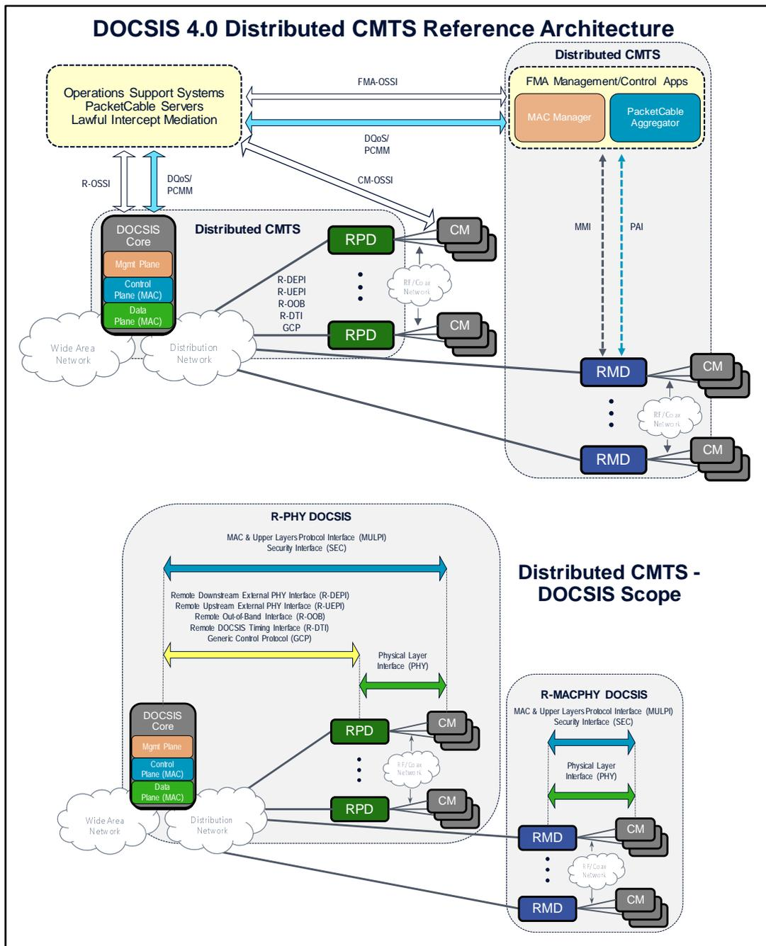
Figure 3: Distributed CMTS reference architecture
