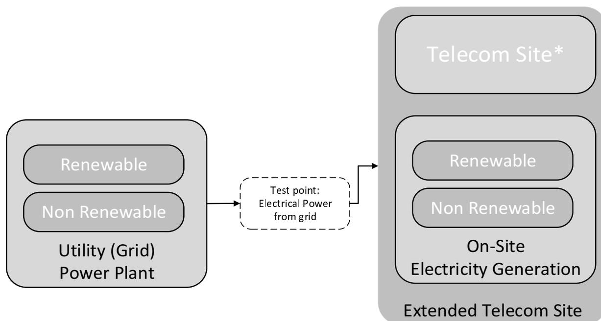
**Figure 3: Schematic representation of the energy sources for a site (the \* refers to the telecommunication Site as in figure 2)**
