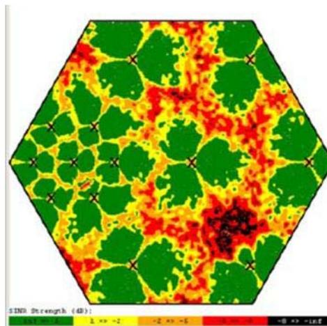
**Figure 4: Typical SINR distribution of a mobile network**
