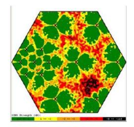
Figure 2: Typical SINR distribution of a mobile network
