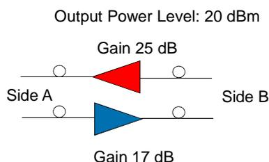
**Figure A.1: Optical amplifier schematic (System Description)**
