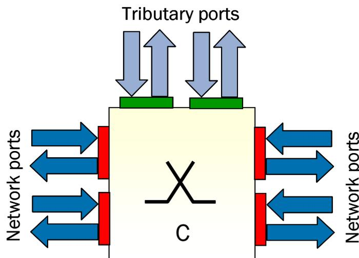
Figure 3: Schematic representation for Category C Transport equipment
