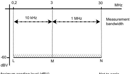
Maximum sending level (dBV) in measurement bandwidth
