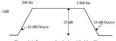
Figure A.1: Response for the band-limiting filter
