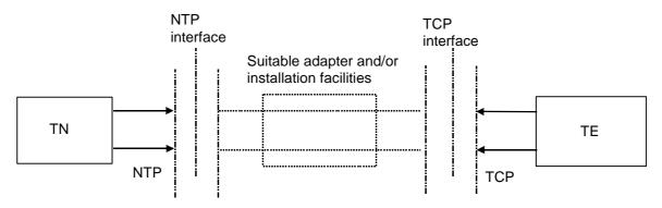
Figure 1: Terminal connection point and network termination point
