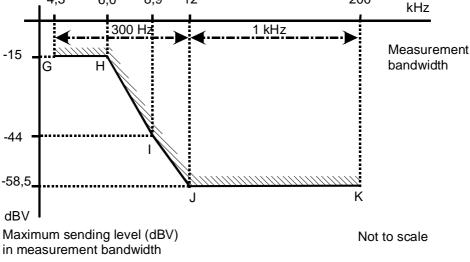
Figure 4: Sending level between 4,3 kHz and 200 kHz
