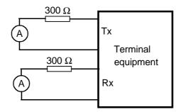
Figure A.11: Power feeding test for 4 wire TE
