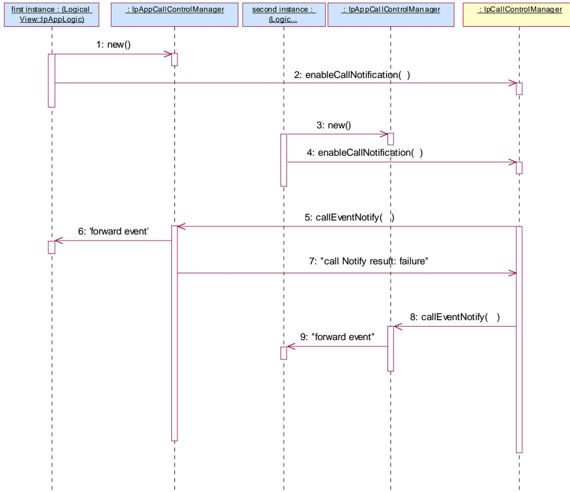
1: The first instance of the application is started on node 1. The application creates a new IpAppCallControlManager to handle callbacks for this first instance of the logic.
