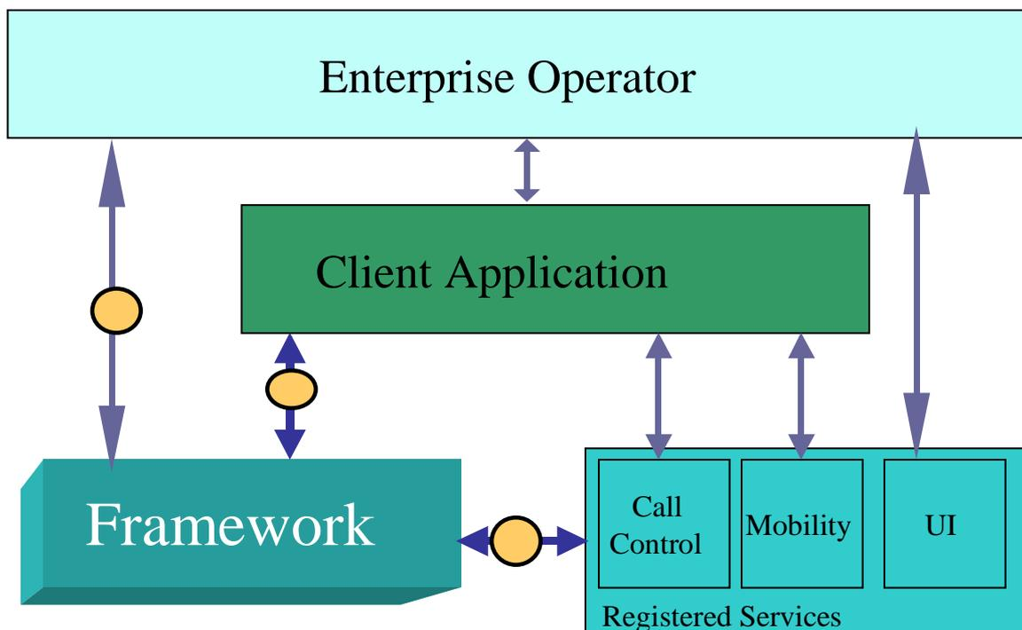
Some of the mechanisms are applied only once (e.g. establishment of service agreement), others are applied each time a user subscription is made to an application (e.g. enabling the call attempt event for a new user).
