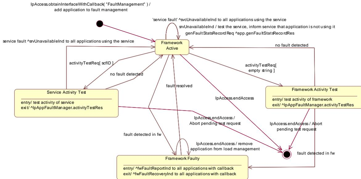
**Figure 17: State Transition Diagram for IpFaultManager**
