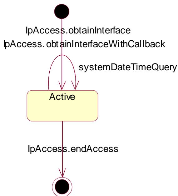
**Figure 16: State Transition Diagram for IpOAM**
