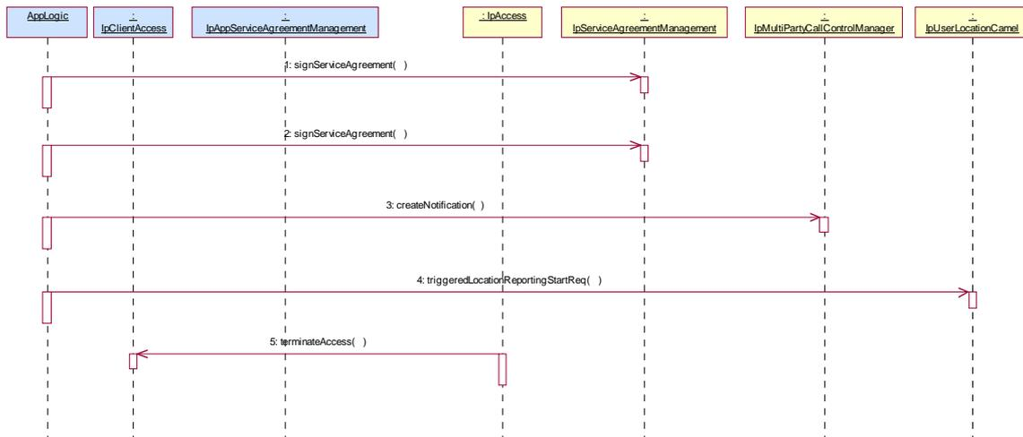
1: Following successful authentication and service discovery, the client initiates the service agreement signing process (not shown). This is completed when the client invokes `signServiceAgreement` on the Framework's `IpServiceAgreementManagement` interface, and a reference to an instance of a service manager interface is returned.
