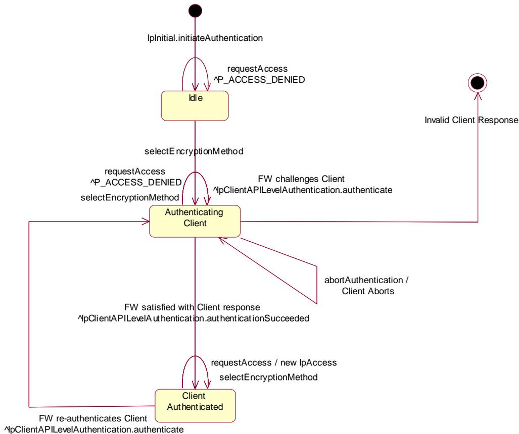
**Figure 5: STD for IpAPILevelAuthentication: Framework authenticates Client using deprecated initiateAuthentication() and authenticate() method combination**
