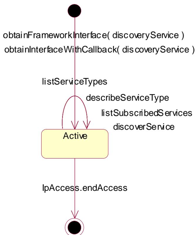
**Figure 18: State Transition Diagram for IpServiceDiscovery**
