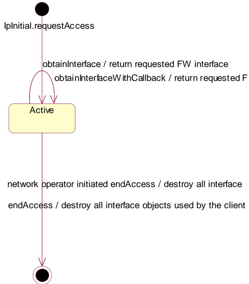
**Figure 7: State Transition Diagram for IpAccess**
