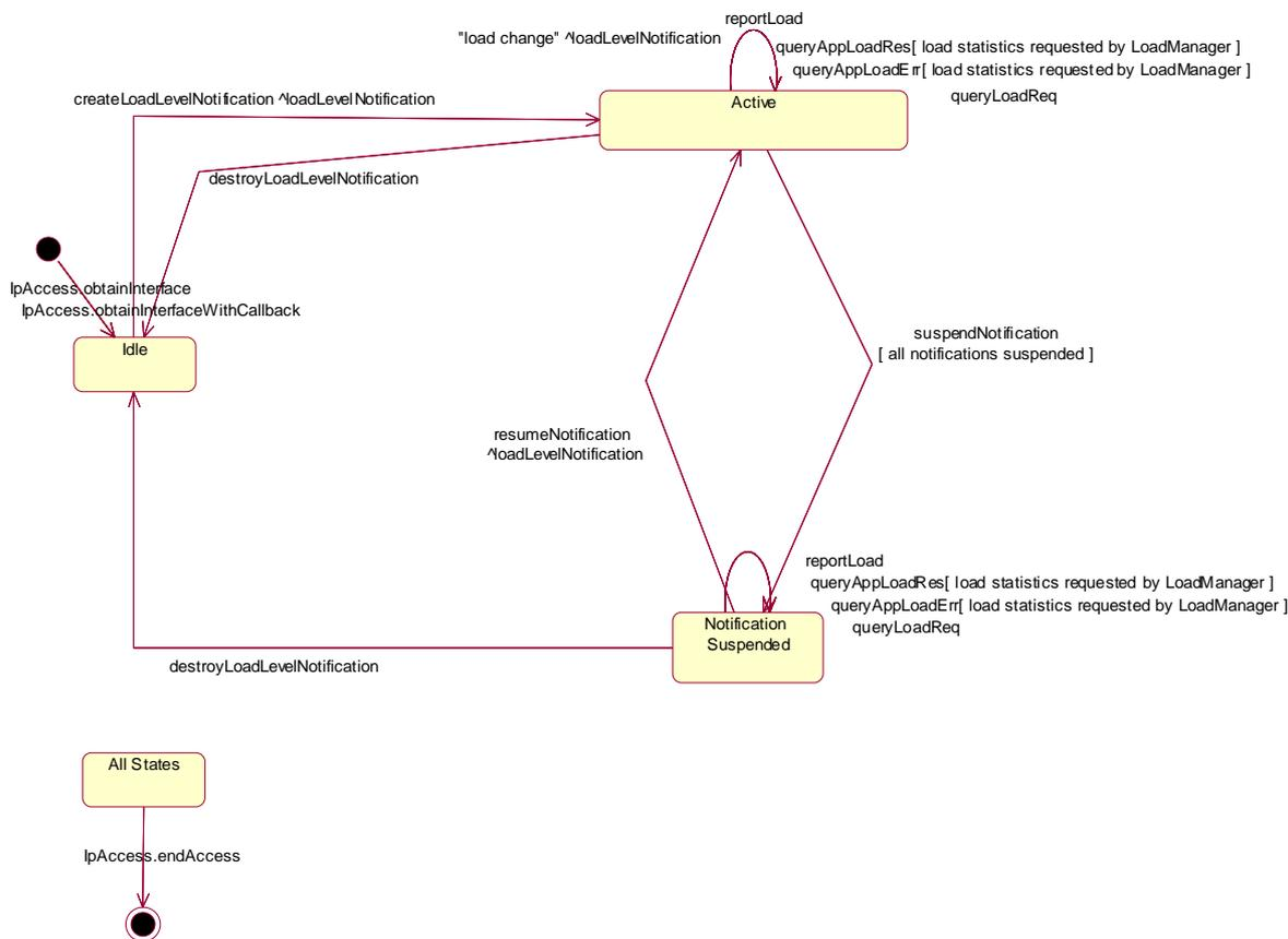
Figure 31: State Transition Diagram for IpFwLoadManager
