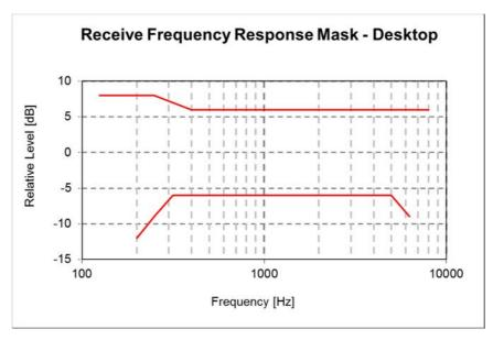
Figure 14: Receive frequency mask for Desktop HFT
