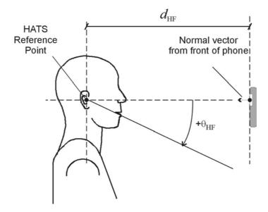
Figure 4: Configuration of Hand-Held loudspeaker relative to the HATS side view
