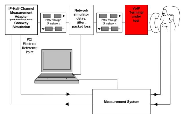
Figure 1: Half channel terminal measurement
