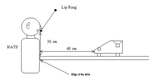
Figure 2: Position for test of desktop hands free terminal side view
