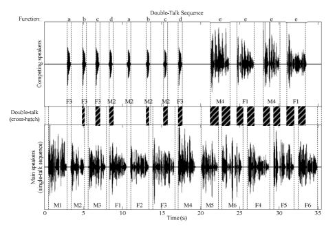
Figure 16: Double talk test sequence with overlapping speech sequences in send and receive direction
