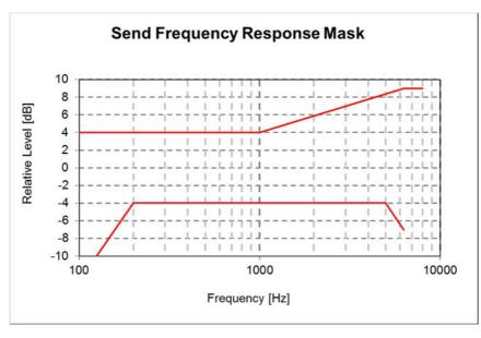
Figure 12: Send sensitivity/frequency mask for HFT
