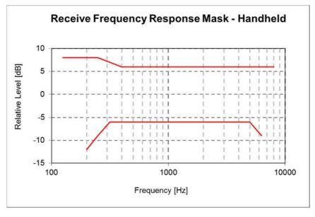
Figure 15: Receive frequency response mask for Hand-held HFT
