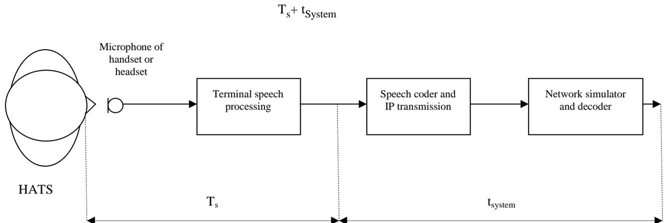
**Figure 8: Different blocks contributing to the delay in send direction**
