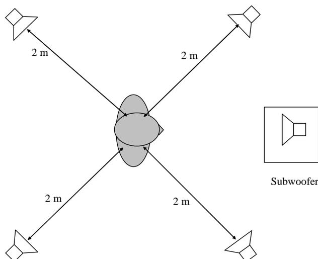
**Figure 2: Loudspeaker arrangement for background noise simulation**
