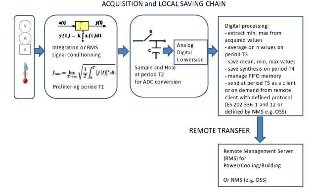
NOTE: The ideal RMS calculation is a mathematical limit at infinite time, but a very precise RMS value may be practically obtained on an integration period much lower than 1 second when the acquisition frequency is of some kHz as achieved by many common integrated chips.
