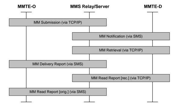
Figure 4: Generalized MMS transaction sequence in fixed networks
