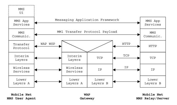
Figure A.2: MM1 protocol layers used in mobile networks today
