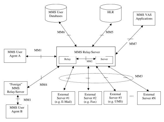
Figure 1: MMS reference architecture
