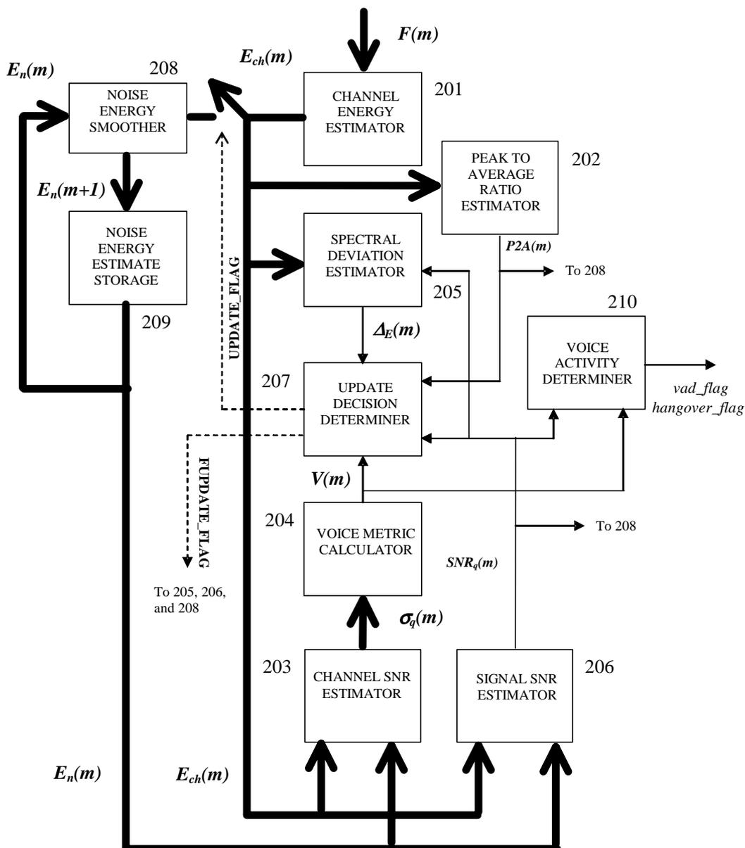
**Figure 5.8: Block diagram of the voice activity detection (VADVC) algorithm**
