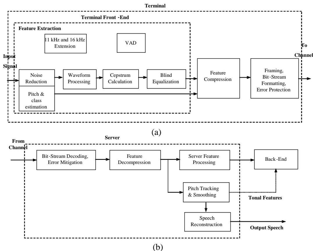
**Figure 4.1: Block scheme of the proposed extended front-end**
