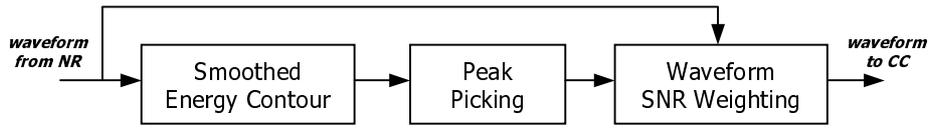
**Figure 5.3: Main components of SNR-dependent waveform processing**
