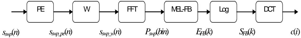
Figure 5.4: Main components of the cepstrum calculation block
