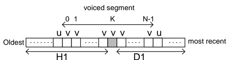
**Figure 10.3: Location of a voiced segment within the first stage buffer**
