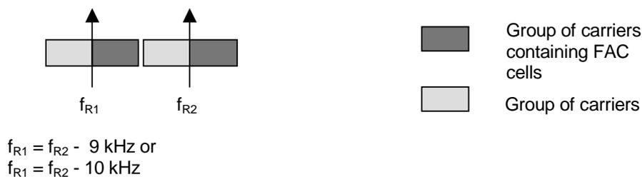
**Figure K.6: Example of base/enhancement DRM signals**
