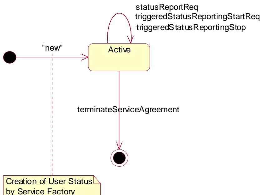
**Figure 6: State Transition Diagram for User Status**
