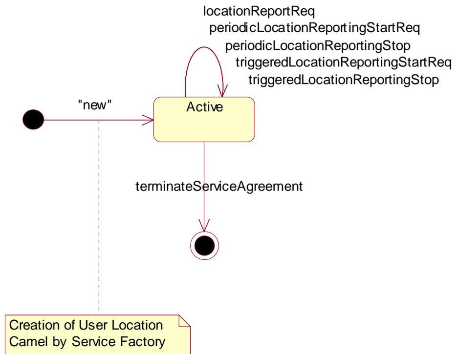
Figure 5: State Transition Diagram for User Location Camel
