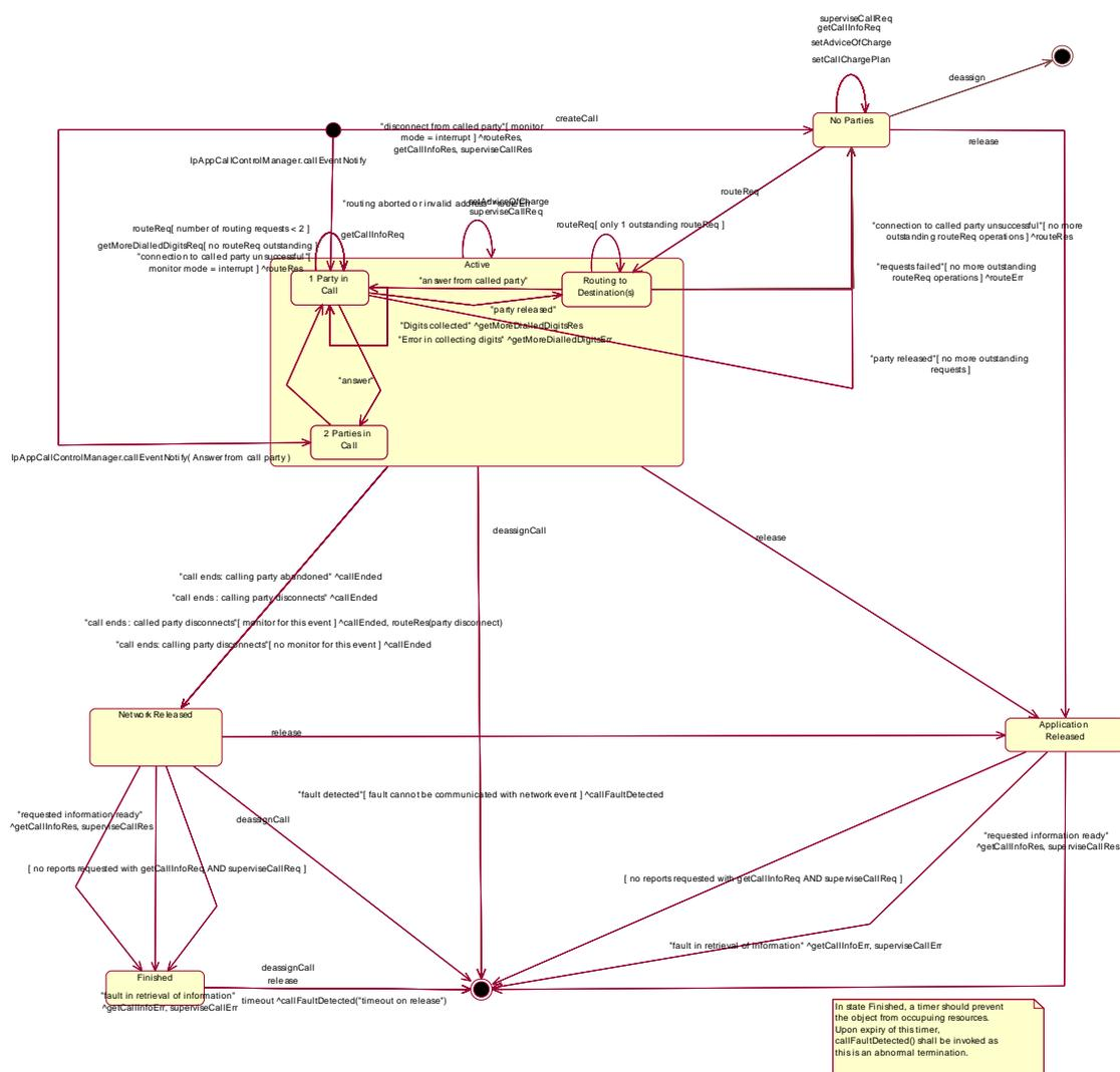
Figure 4: Application view on the IpCall object
