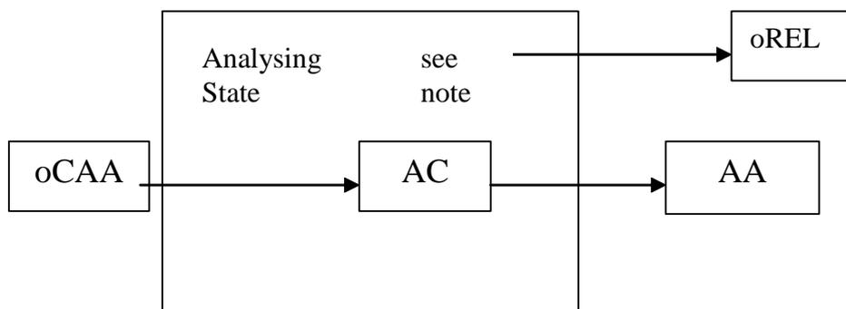
NOTE: The release event (oREL) can occur in any state resulting in a transition to Releasing state.
