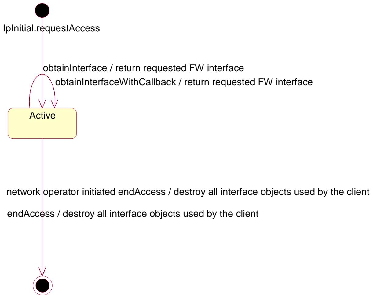
**Figure 4: State Transition Diagram for IpAccess**
