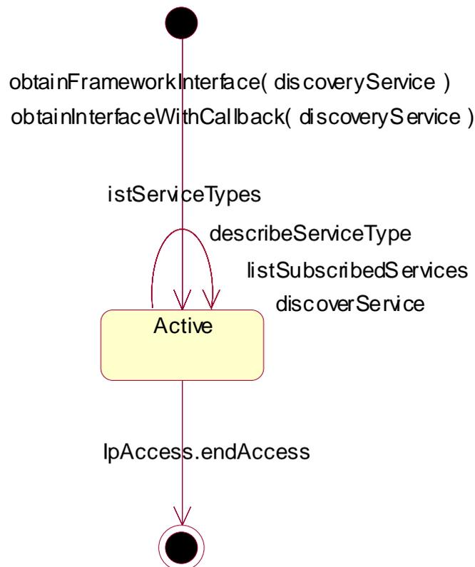
**Figure 10: State Transition Diagram for IpServiceDiscovery**
