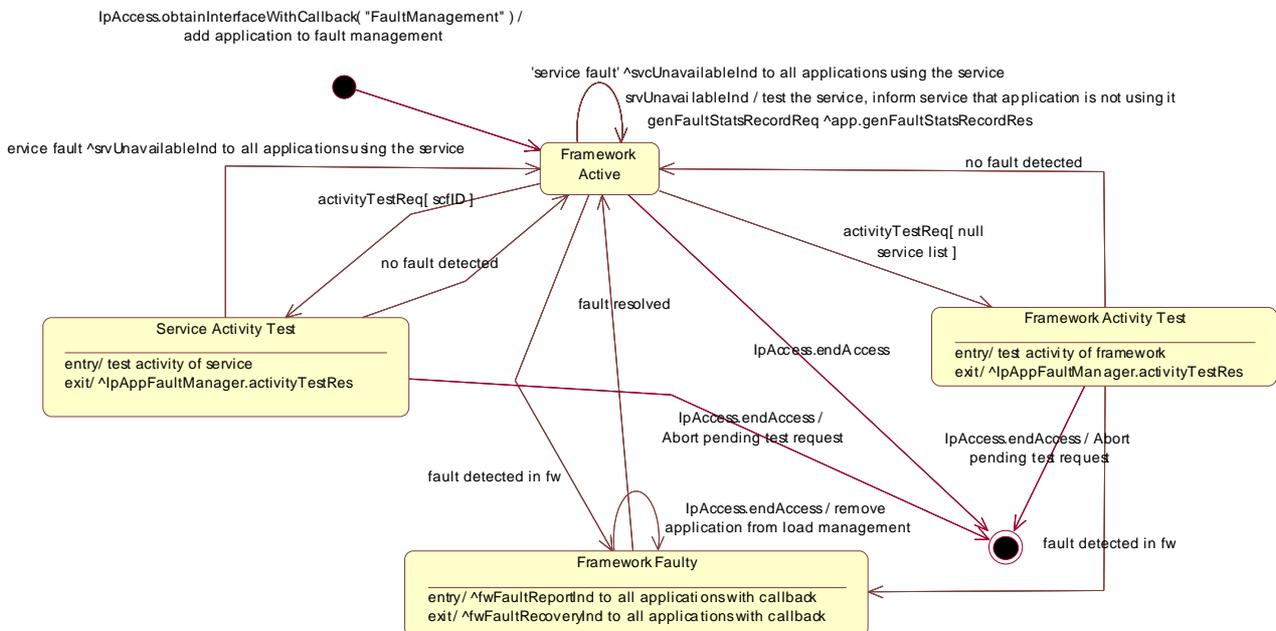
Figure 14: State Transition Diagram for IpFaultManager
