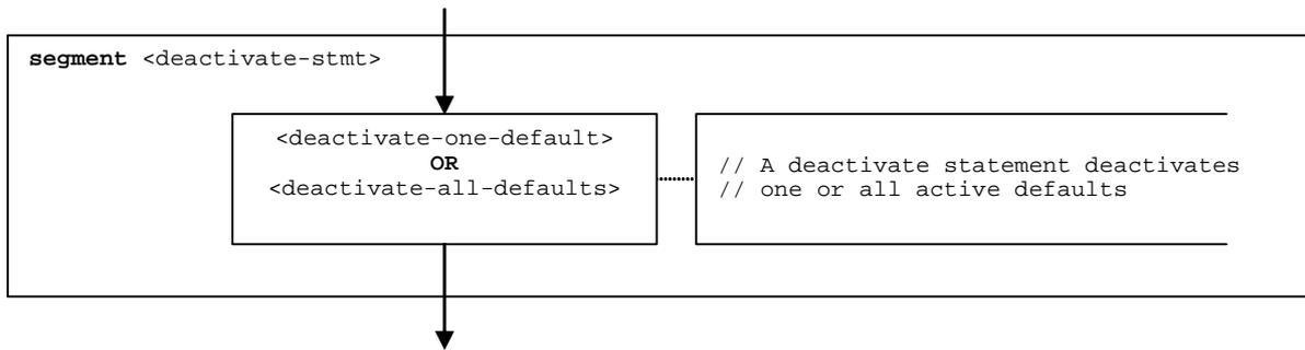
Figure 63a: Flow graph segment `<deactivate-stmt>`
