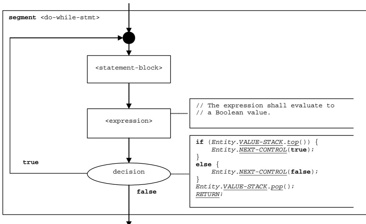
Figure 65: Flow graph segment `<do-while-stmt>`
