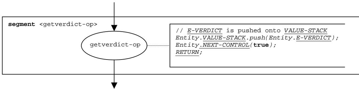
Figure 88: Flow graph segment `<getverdict-op>`
