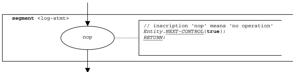
Figure 92: Flow graph segment <log-stmt>
