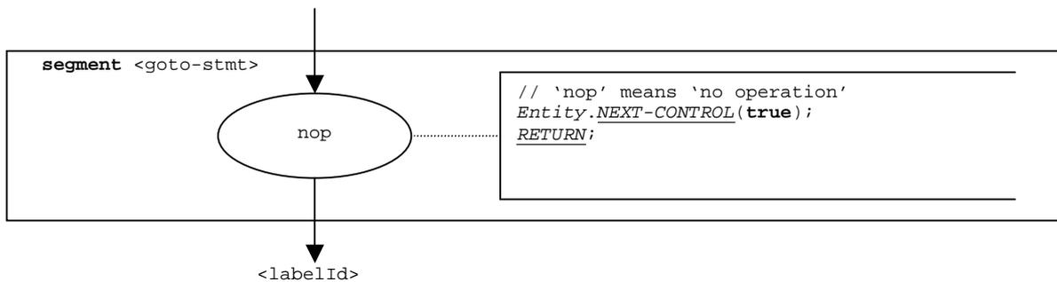
Figure 89: Flow graph segment `<goto-stmt>`
