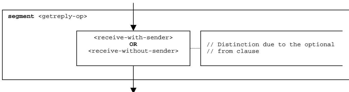
Figure 87: Flow graph segment `<getreply-op>`
