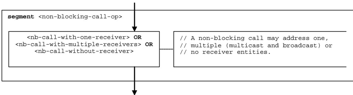
Figure 48: Flow graph segment <non-blocking-call-op>
