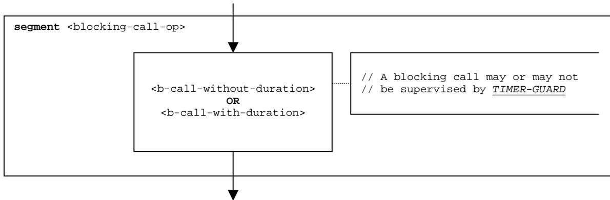
Figure 47: Flow graph segment <blocking-call-op>
