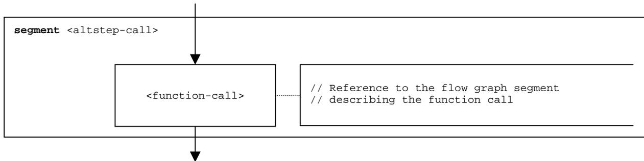
Figure 44: Flow graph segment <altstep-call>
