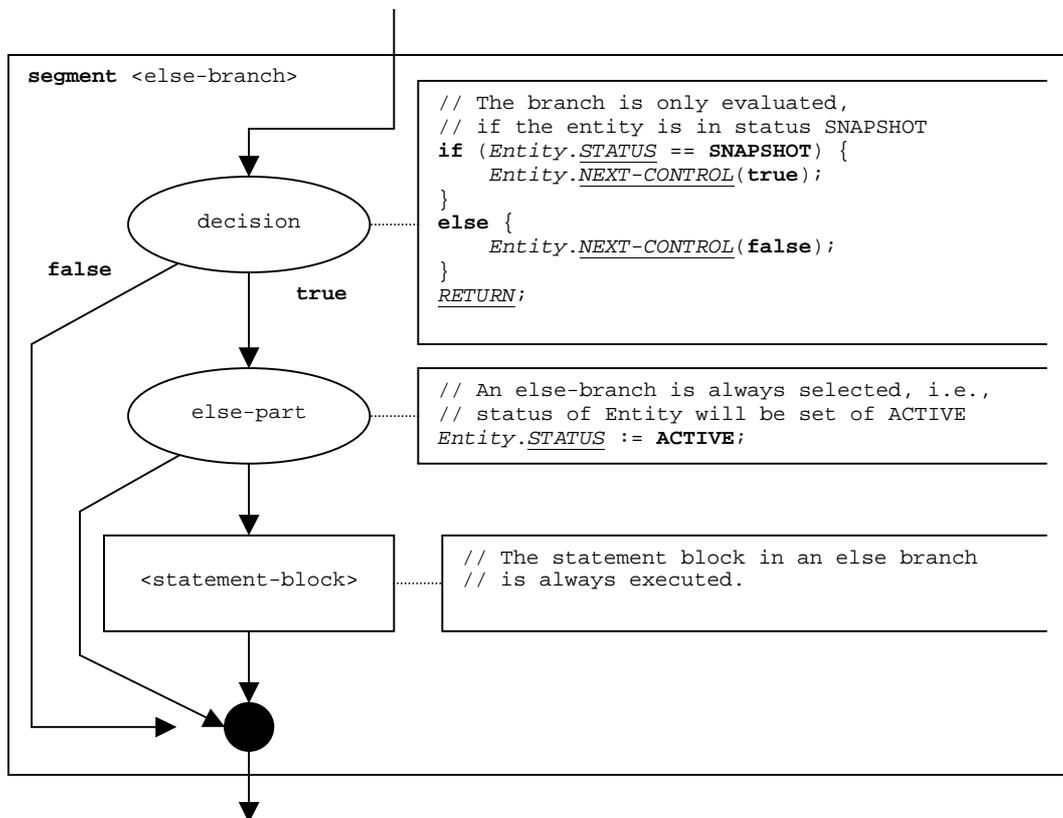
Figure 42: Flow graph segment <else-branch>
