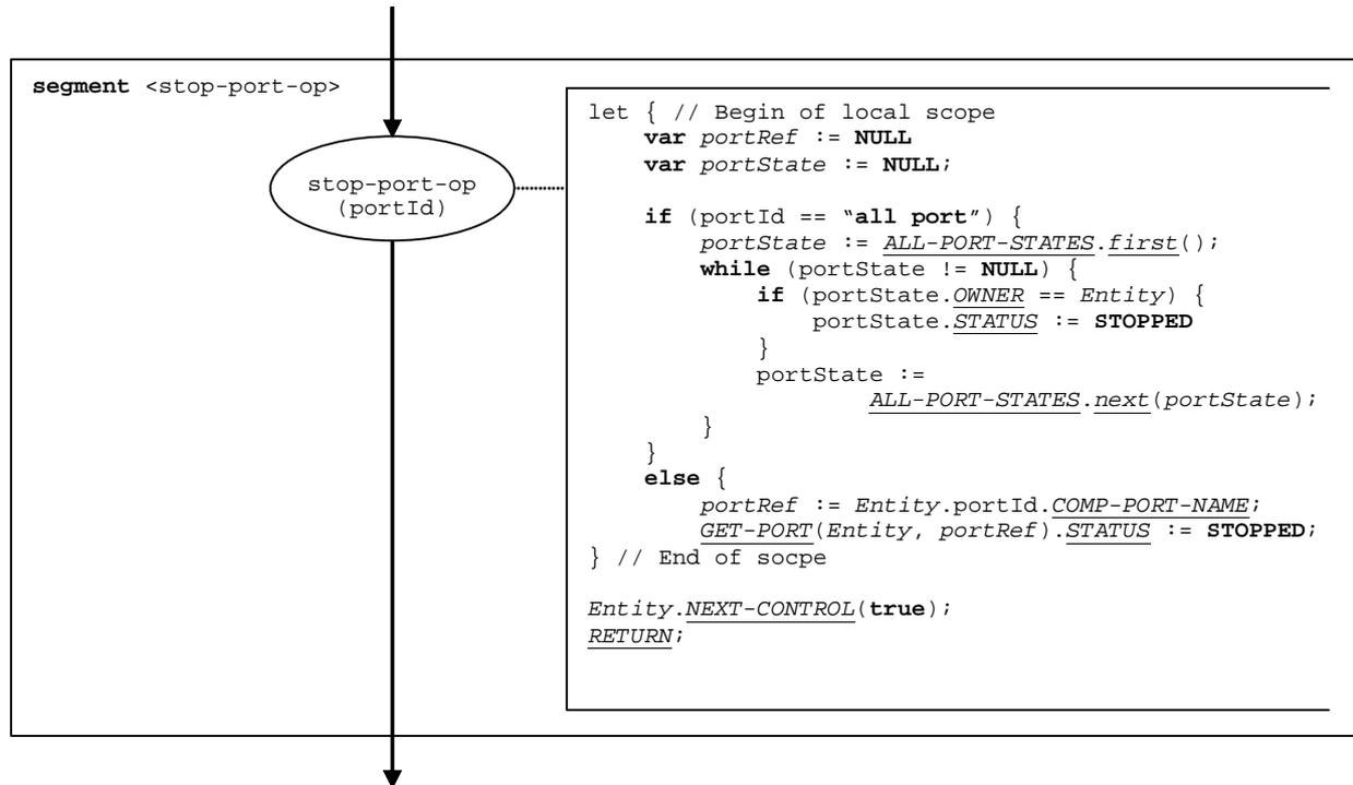
Figure 129: Flow graph segment <stop-port-op>
