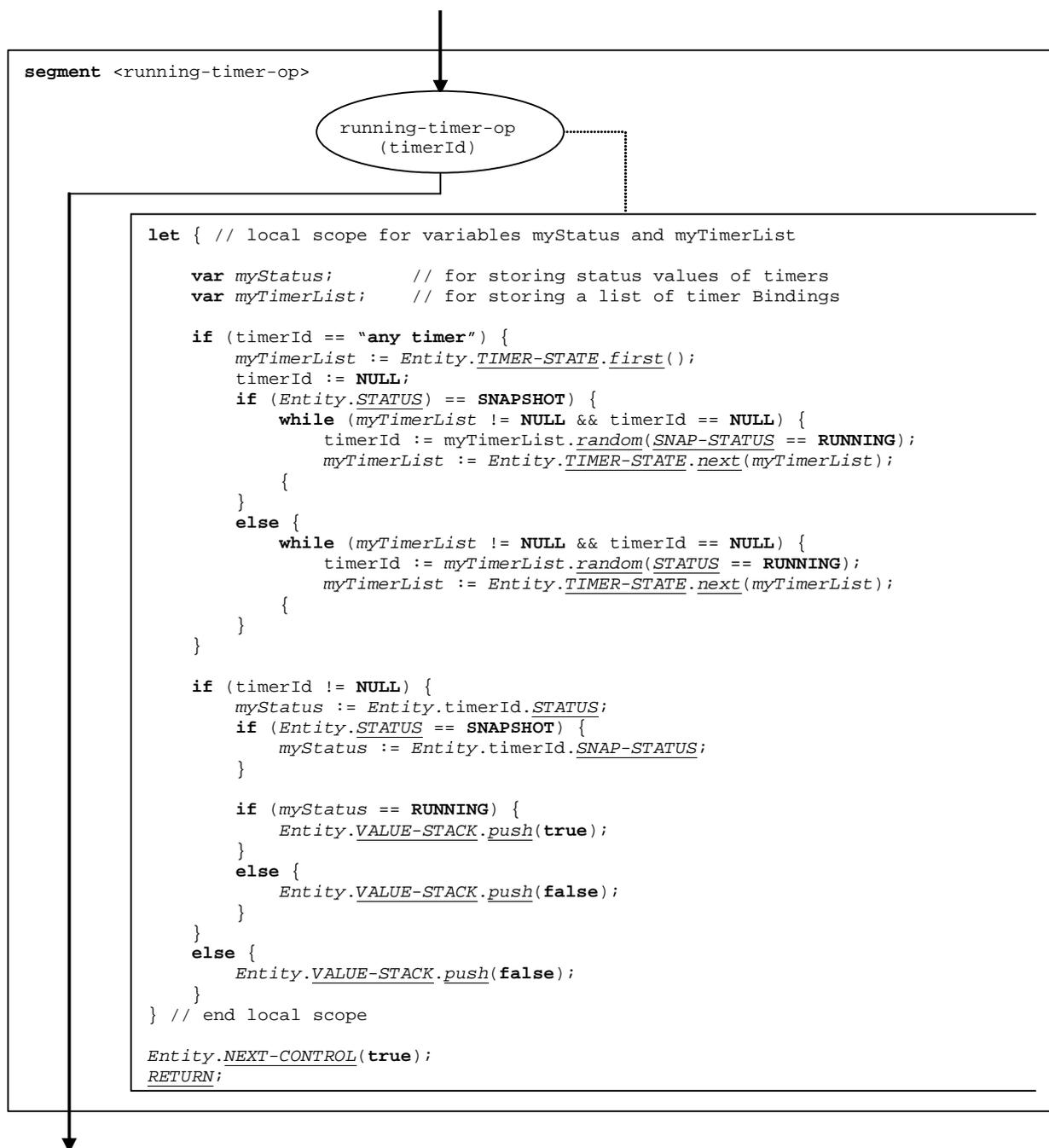
Figure 114: Flow graph segment <running-timer-op>
