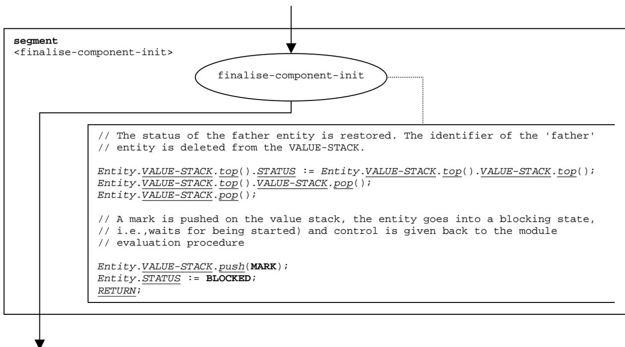
Figure 75: Flow graph segment <finalise-component-init>
