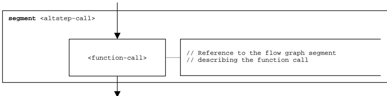
Figure 44: Flow graph segment <altstep-call>
