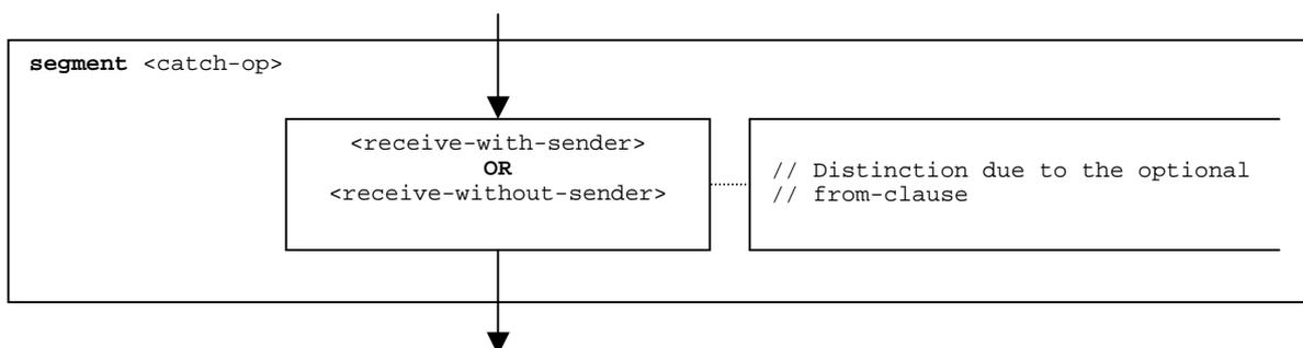
Figure 55: Flow graph segment <catch-op>
