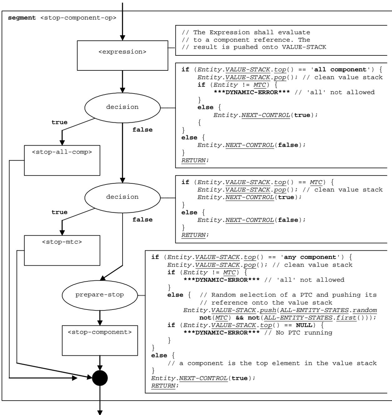
Figure 125: Flow graph segment <stop-component-op>
