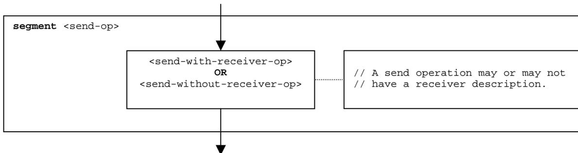
Figure 116: Flow graph segment `<send-op>`
