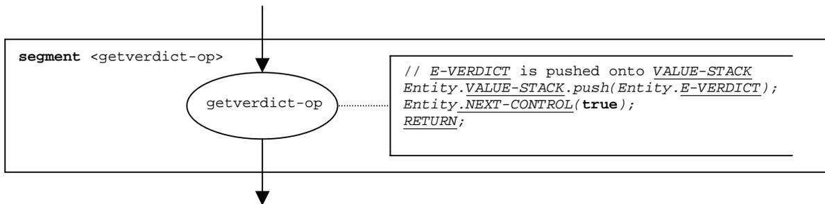
Figure 88: Flow graph segment `<getverdict-op>`
