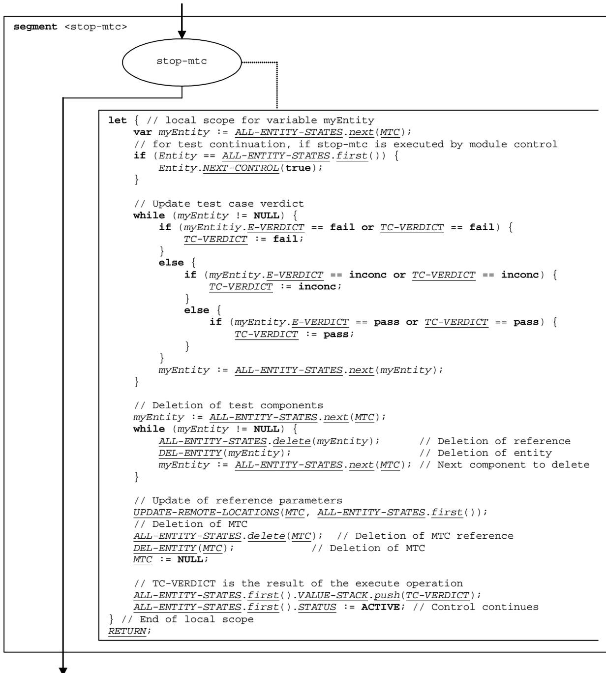
Figure 126: Flow graph segment <stop-mtc-op>
