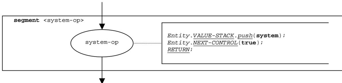
Figure 133: Flow graph segment <system-op>
