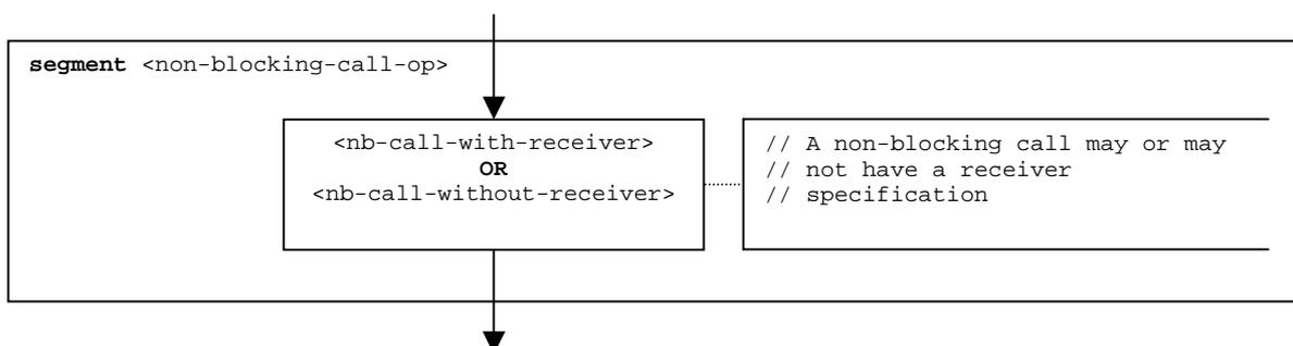
Figure 48: Flow graph segment <non-blocking-call-op>
