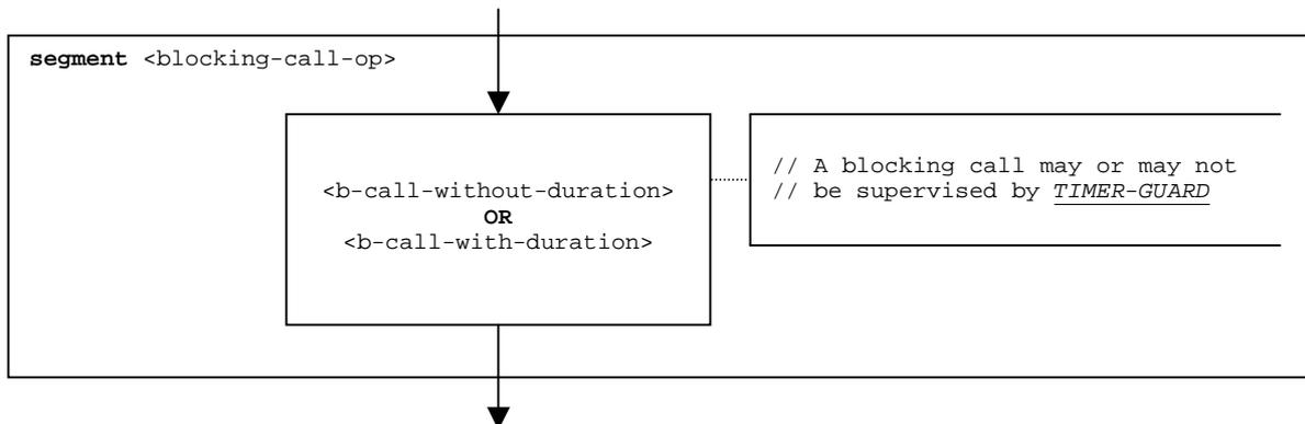
Figure 47: Flow graph segment <blocking-call-op>
