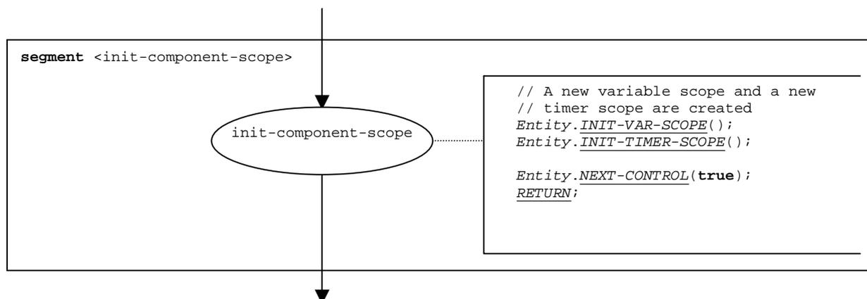
Figure 76: Flow graph segment <init-component-scope>
