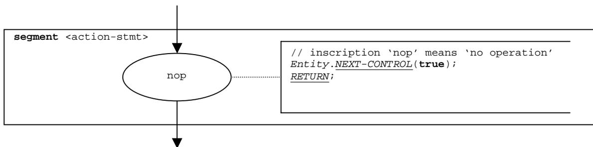
Figure 36: Flow graph segment <action-stmt>
