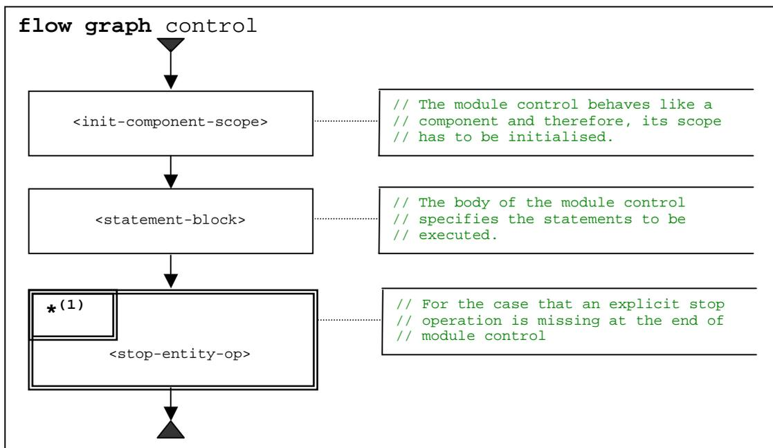
Figure 18: Flow graph representation of module control
