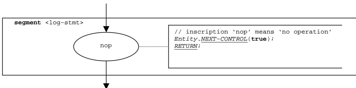
**Figure 92: Flow graph segment <log-stmt>**
