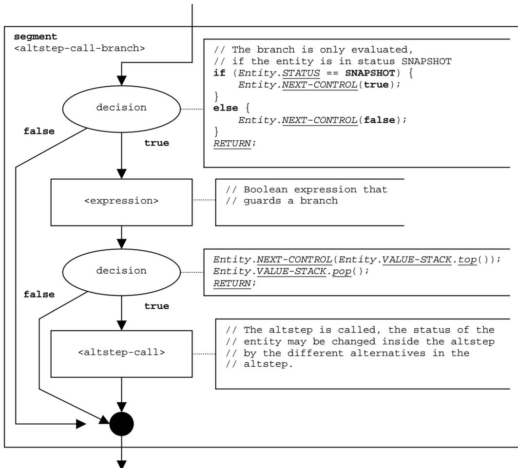
Figure 41: Flow graph segment <altstep-call-branch>
