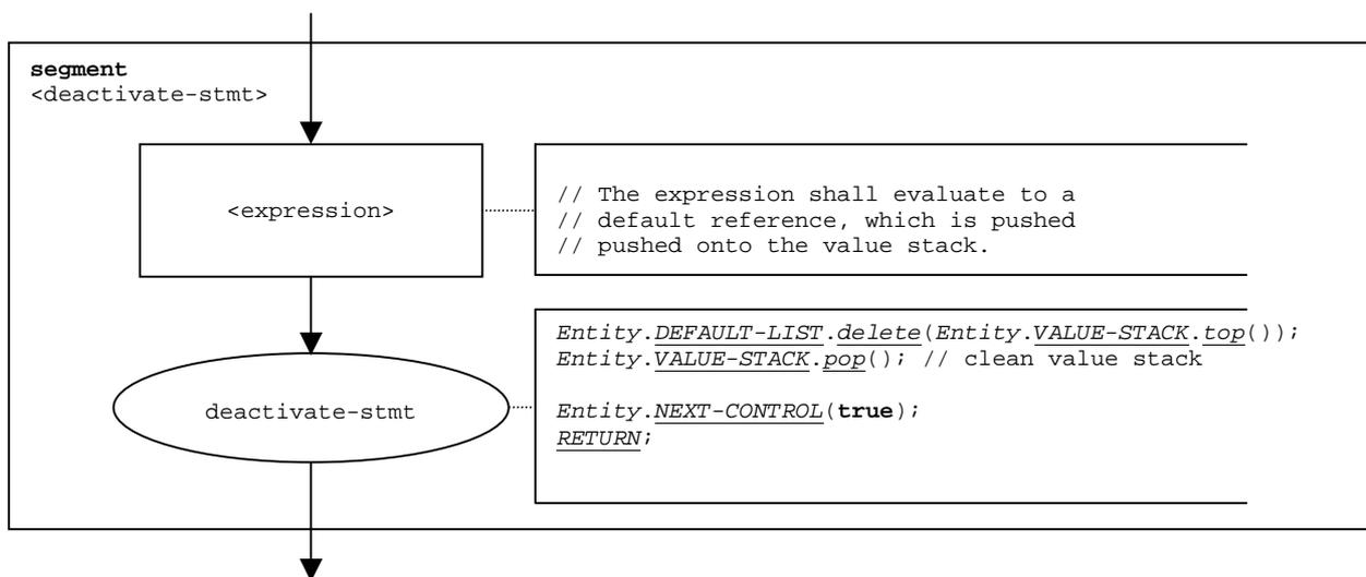
Figure 63: Flow graph segment <deactivate-stmt>
