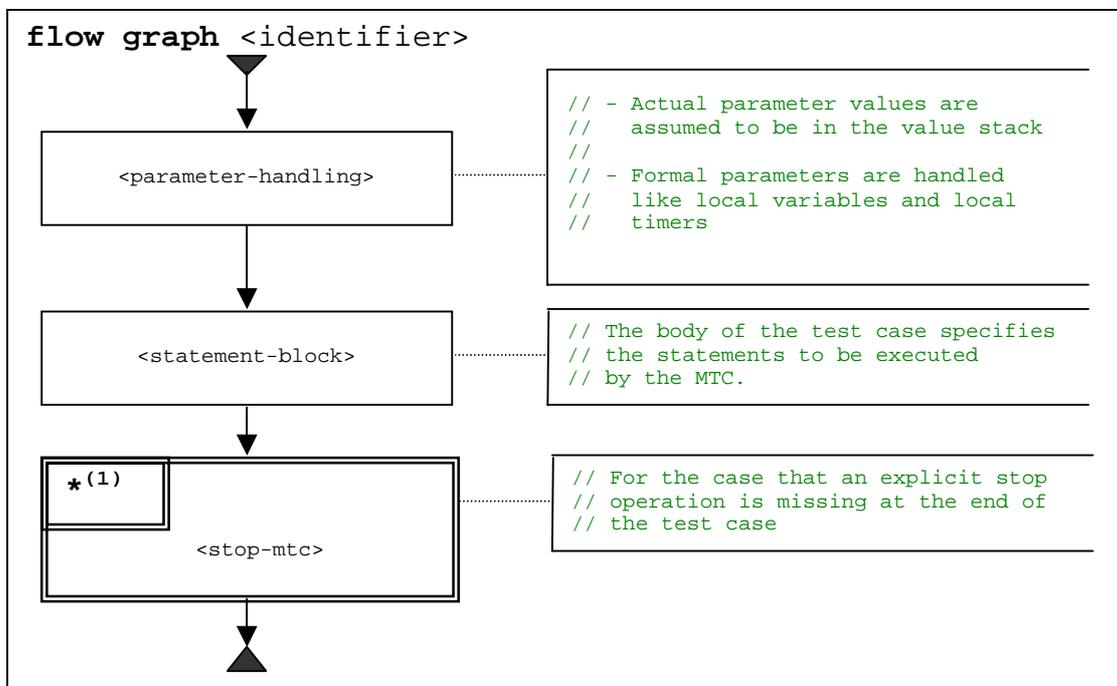
Figure 19: Flow graph representation of test cases
