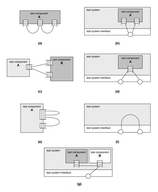
Figure 7: NOT allowed connections
