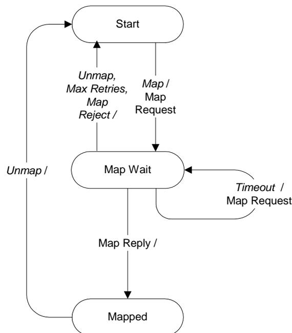
**Figure 8.1: SA mapping state machine flow diagram**
