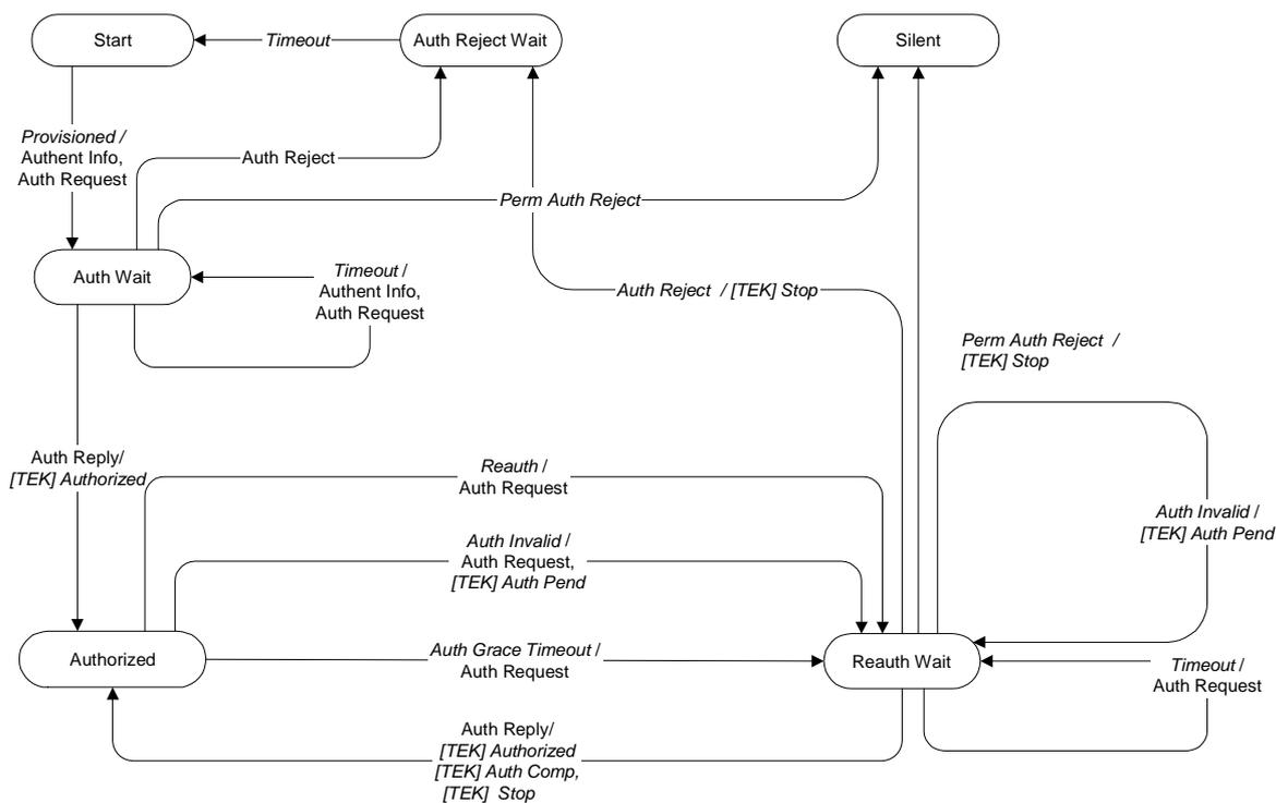
Figure 7.1: Authorization state machine flow diagram
