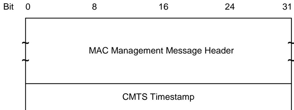
**Figure 8-15: Format of Packet PDU Following the Timing Header**
