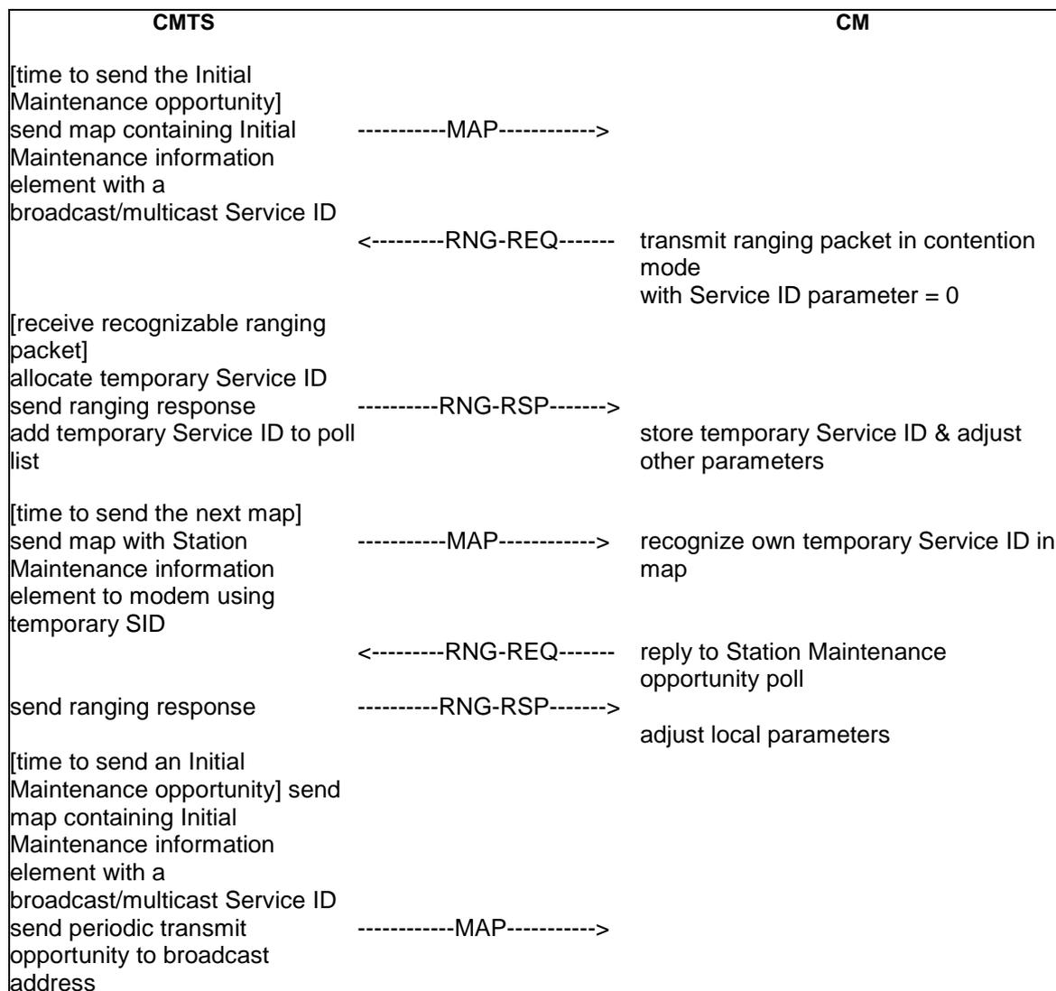
**Figure 11-5: Ranging and Automatic Adjustments Procedure**
