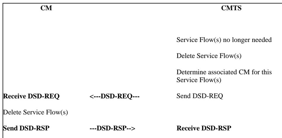
**Figure 11-51: Dynamic Service Deletion Initiated from CMTS**
