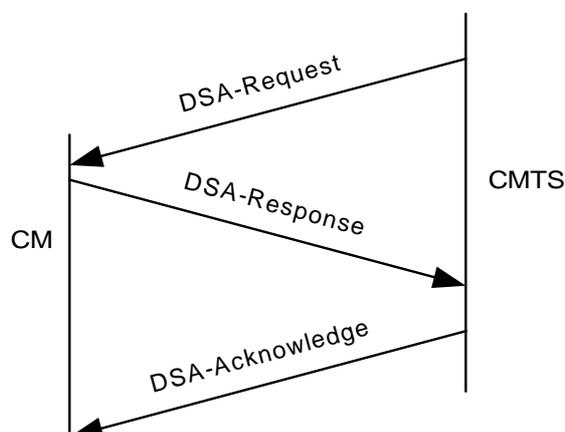
**Figure 10-7: Dynamic Service Addition Message Flow - CMTS Initiated**
