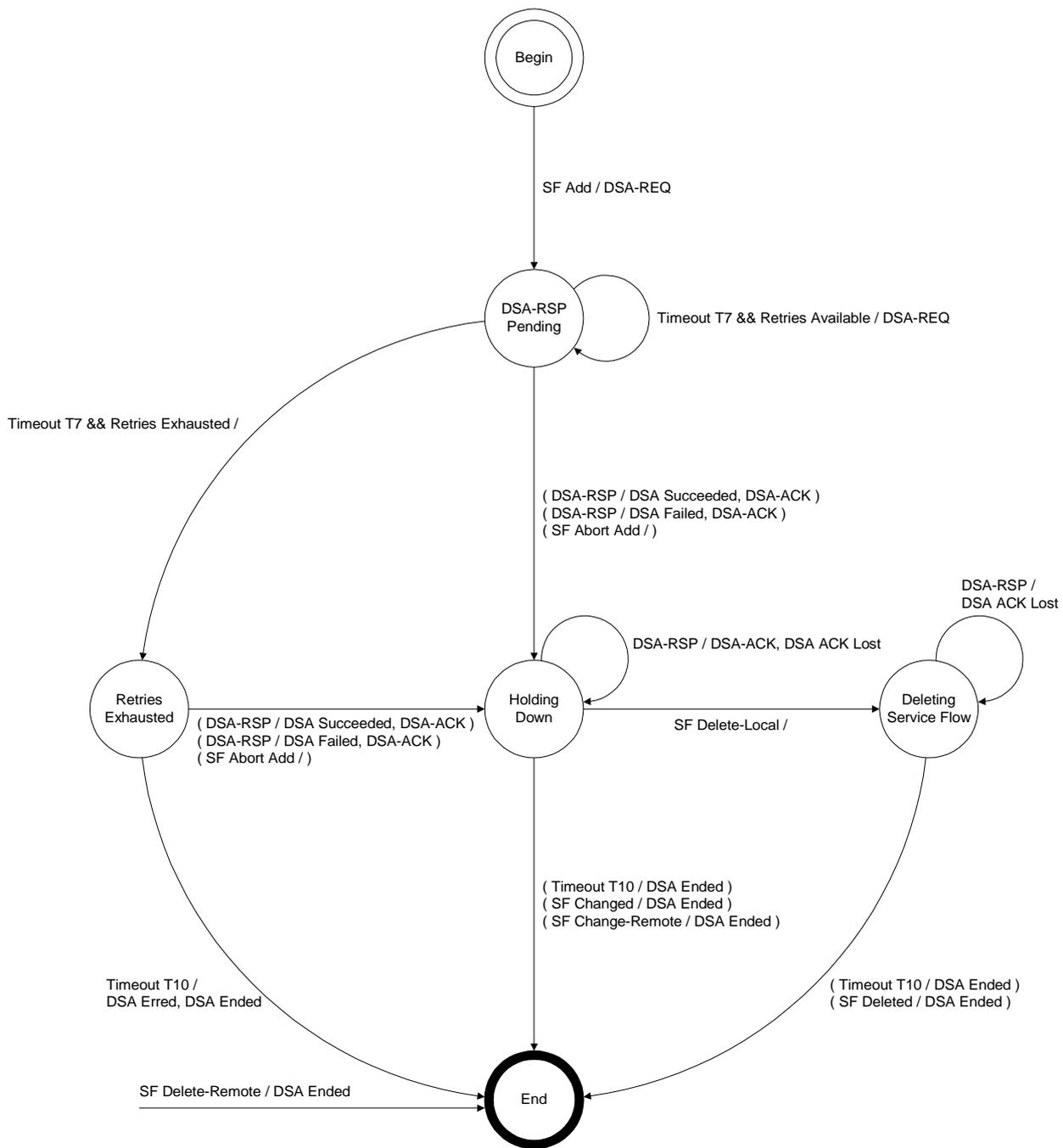
Figure 11-22: DSA-locally Initiated Transaction State Transition Diagram
