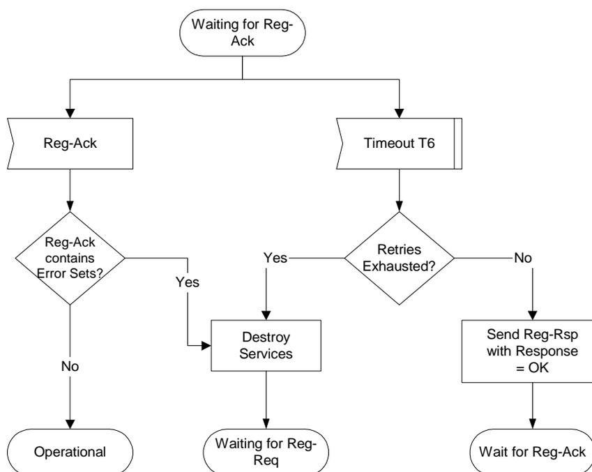
Figure 11-15: Registration Acknowledgment- CMTS
