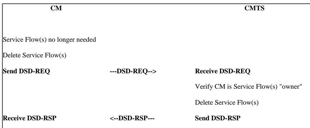
**Figure 11-50: Dynamic Service Deletion Initiated from CM**
