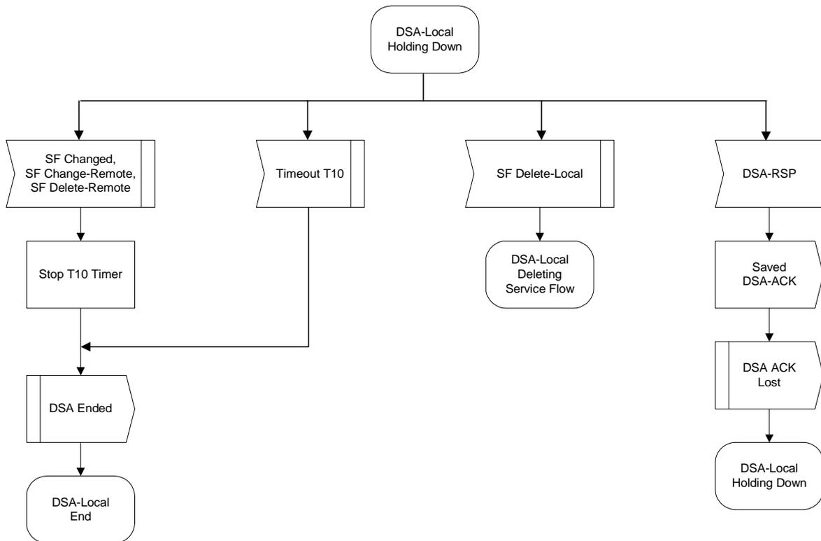
Figure 11-32: DSA-Locally Initiated Transaction Holding State Flow Diagram
