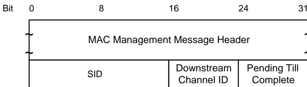
Figure 8-21: Packet PDU Following the Timing Header
