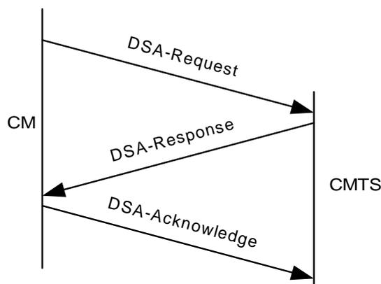
**Figure 10-6: Dynamic Service Addition Message Flow - CM Initiated**
