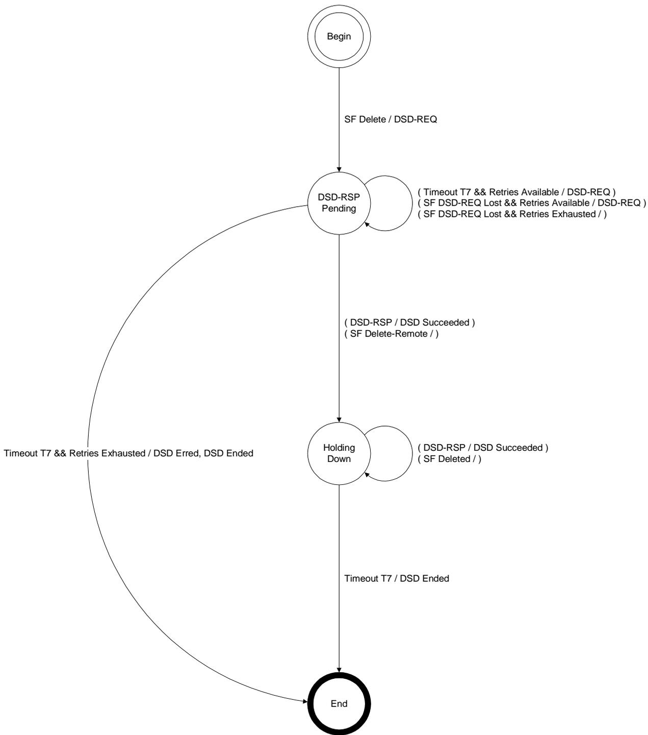
Figure 11-26: DSD-Locally Initiated Transaction State Transition Diagram
