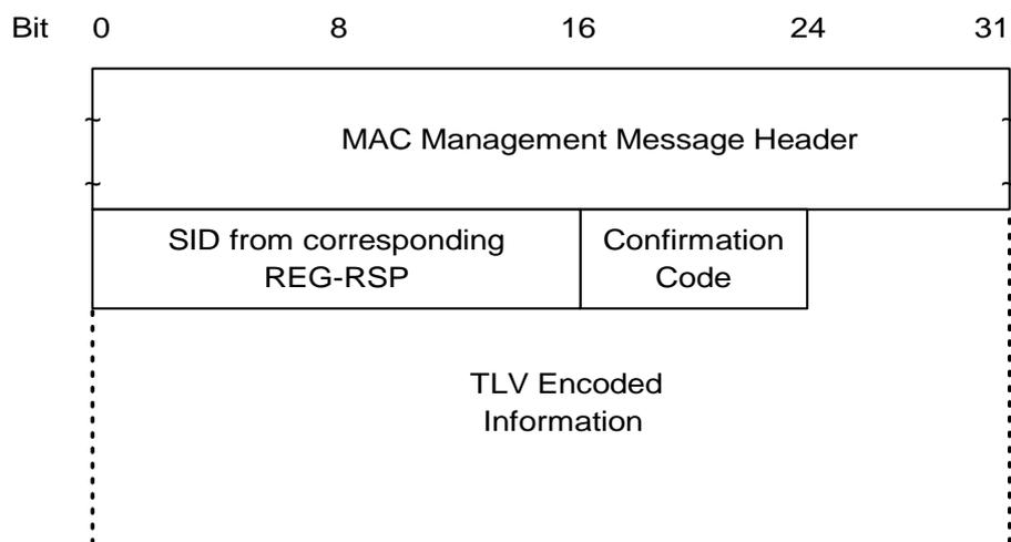
**Figure 8-28: Registration Acknowledgment**
