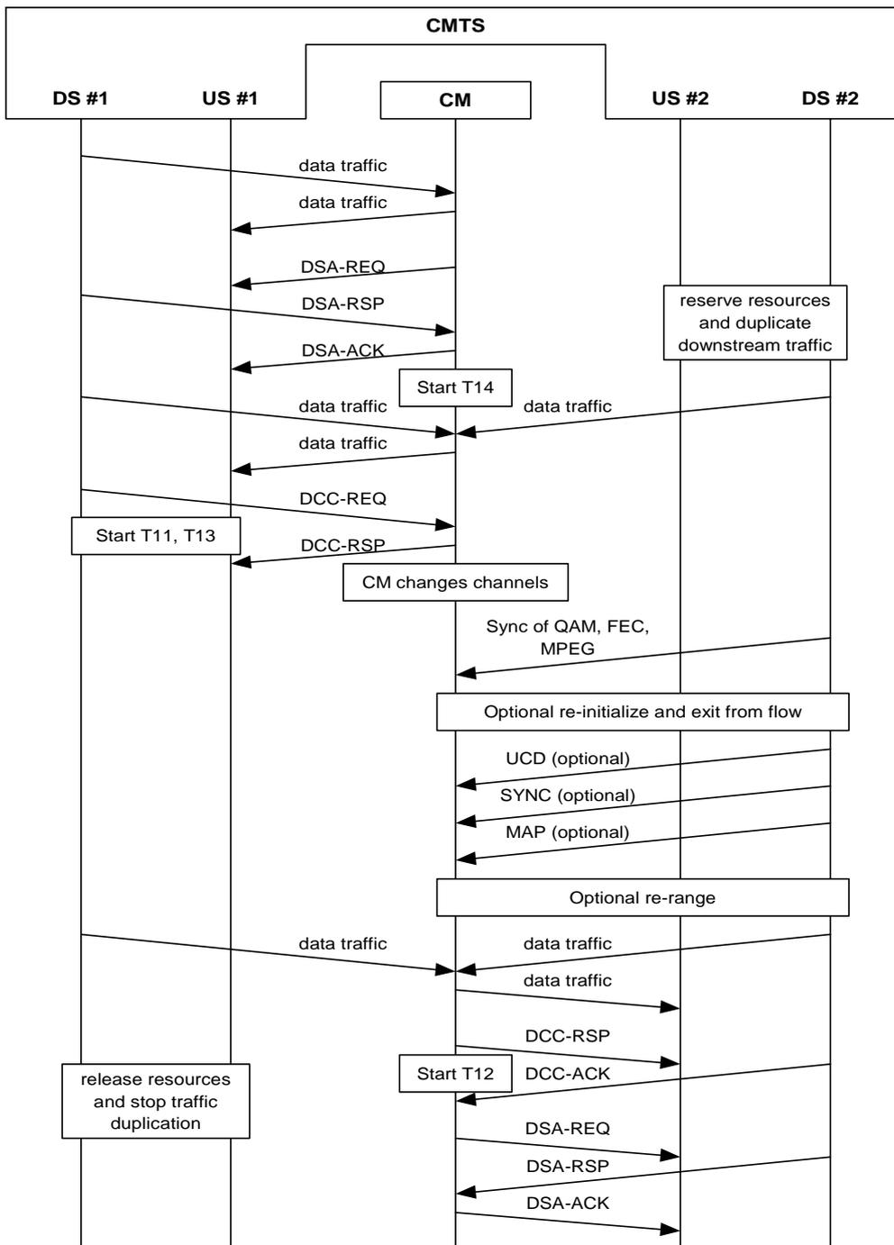
**Figure 11-57: DCC Example Operational Flow**
