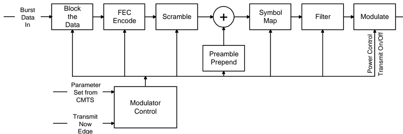
Figure 6-9: Signal-Processing Sequence
