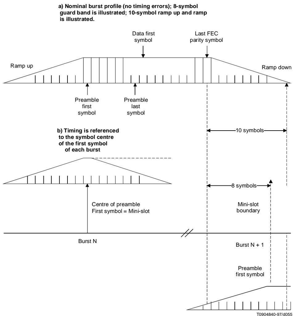
NOTE – Ramp down of one burst can overlap ramp up of following burst even with one transmitter assigned both bursts.
