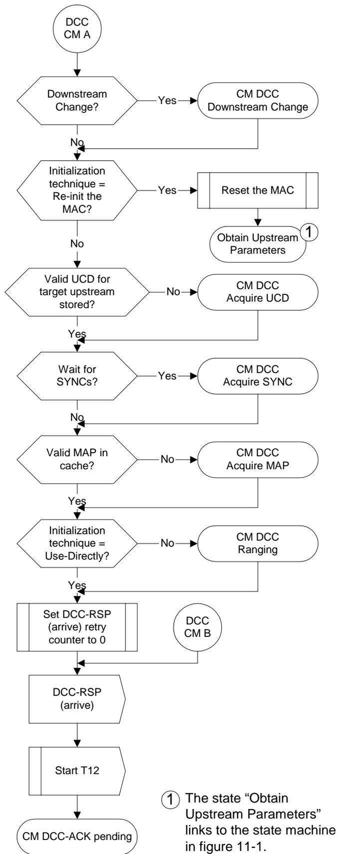
Figure 11-63: Dynamically Changing Channels: CM View Part 2
