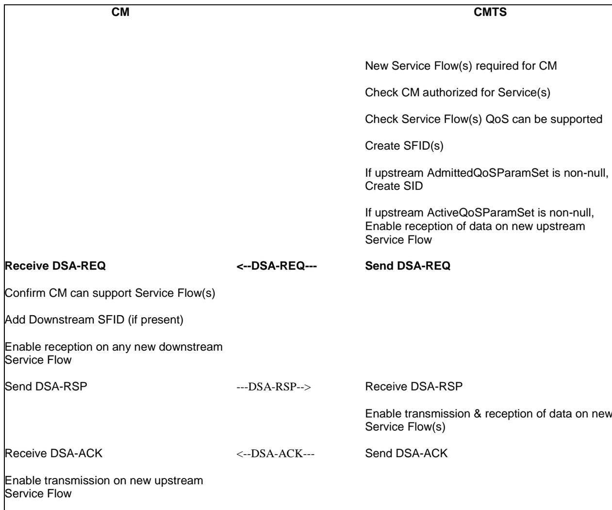
**Figure 11-29: Dynamic Service Addition Initiated from CMTS**
