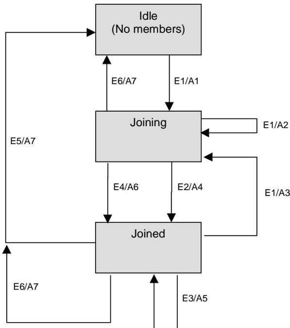
**Figure L-1: IGMP Support - CM passive mode**
