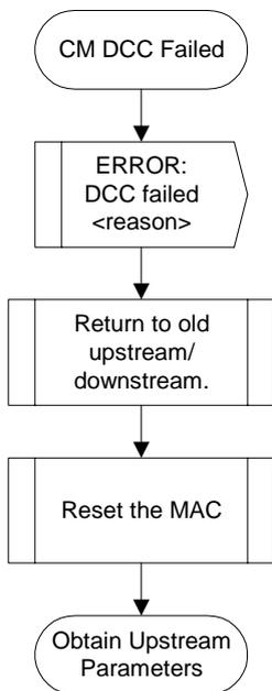
The state "Obtain Upstream Parameters" links to the state machine in figure 11-1.
