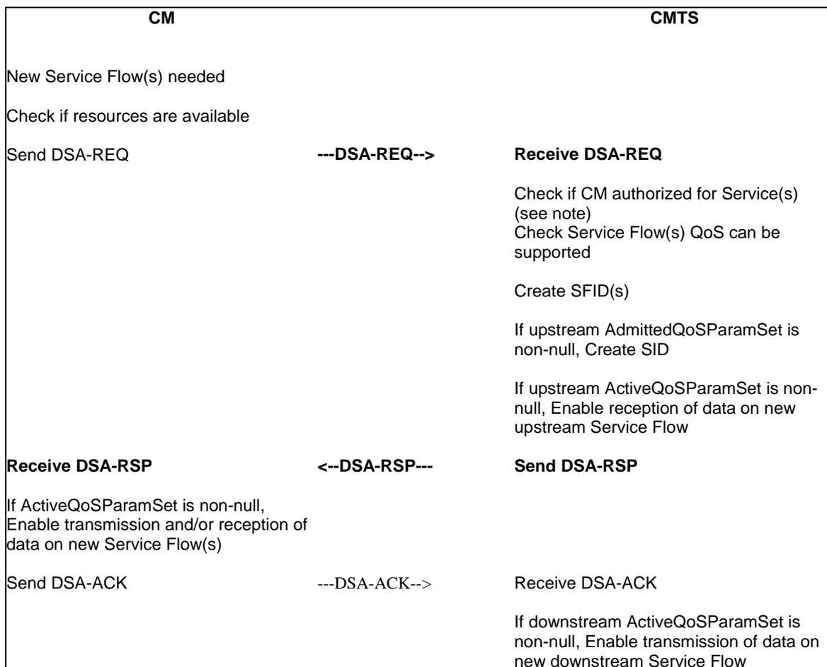
NOTE: Authorization can happen prior to the DSA-REQ being received by the CMTS. The details of CMTS signalling to anticipate a DSA-REQ are beyond the scope of the present document.
