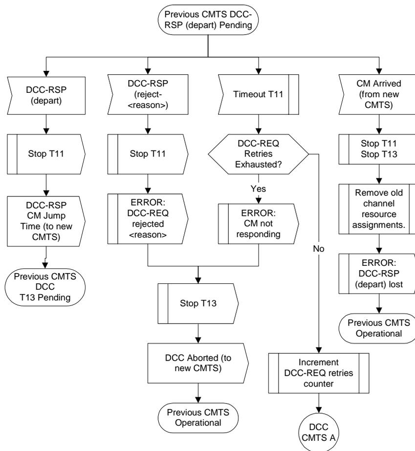
Figure 11-59: Dynamically Changing Channels: CMTS View Part 2
