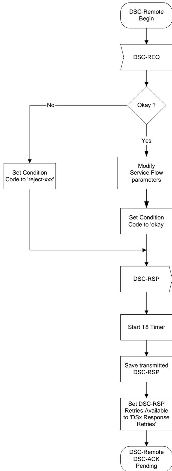
Figure 11-46: DSC-Remotely Initiated Transaction Begin State Flow Diagram
