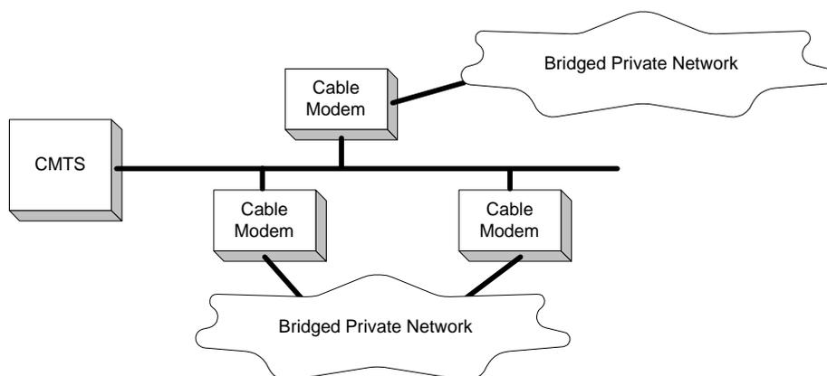
**Figure I-1: Spanning Tree Topology**
