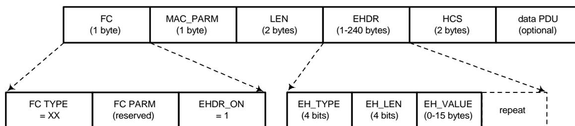
**Figure 8-12: Extended MAC Format****Table 8-11: Example Extended Header Format**
