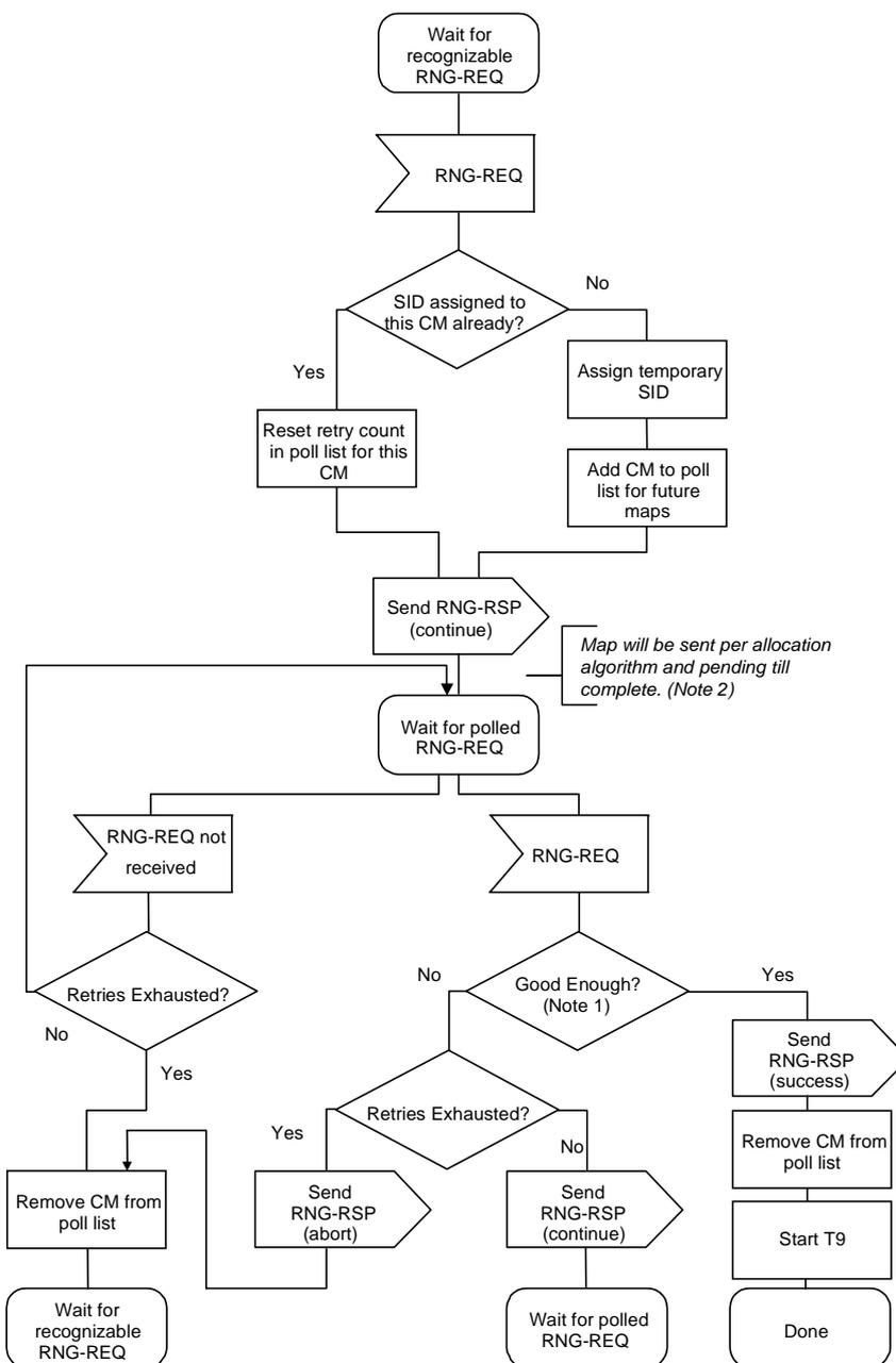
NOTE 1: Means ranging is within the tolerable limits of the CMTS.
