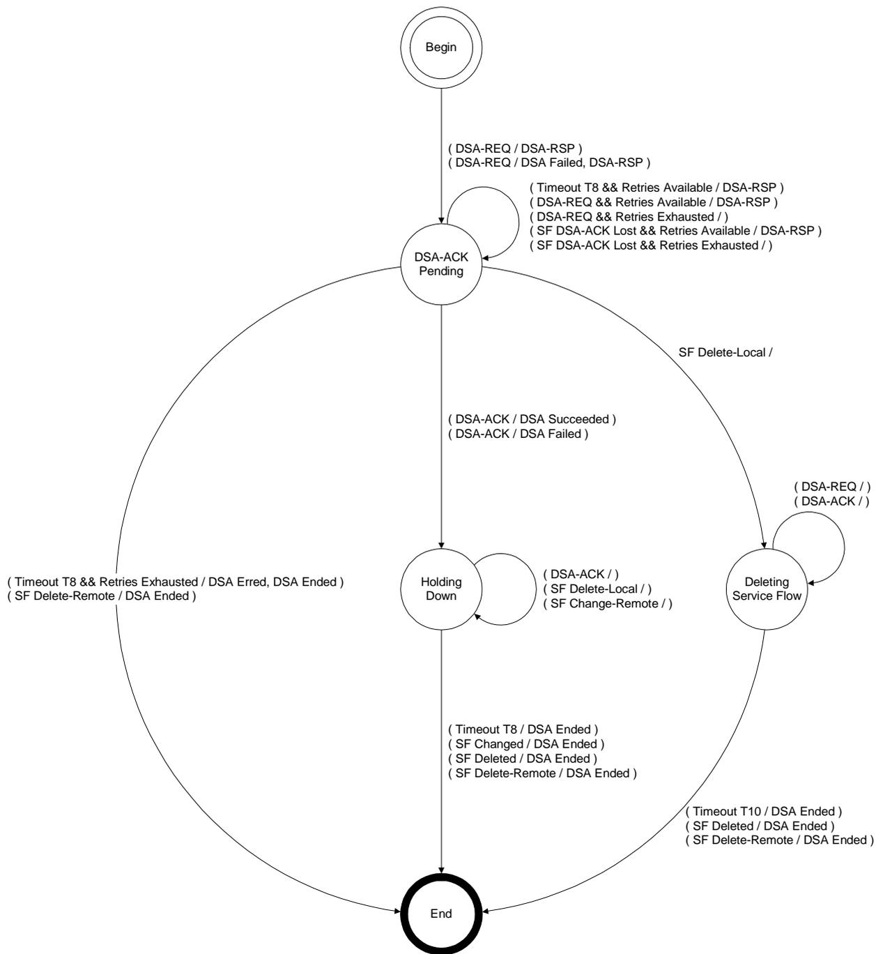
Figure 11-23: DSA-Remotely Initiated Transaction State Transition Diagram
