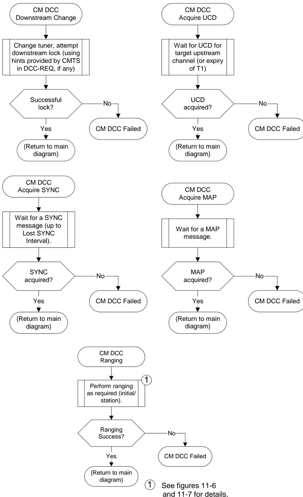
Figure 11-64: Dynamically Changing Channels: CM View Part 3
