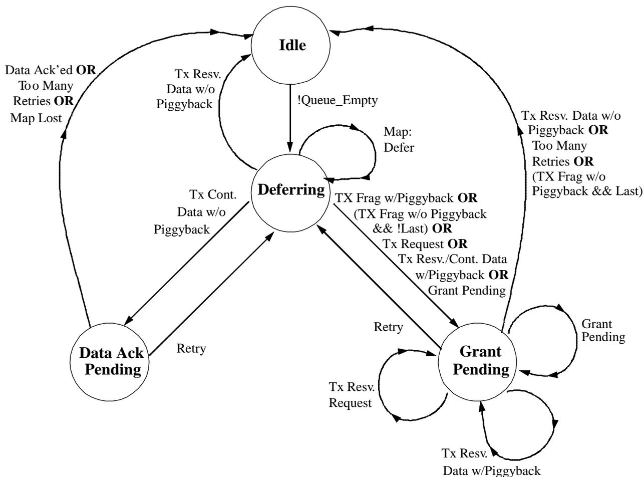
**Figure K-1: Transmission & Deference State Transition Diagram**
