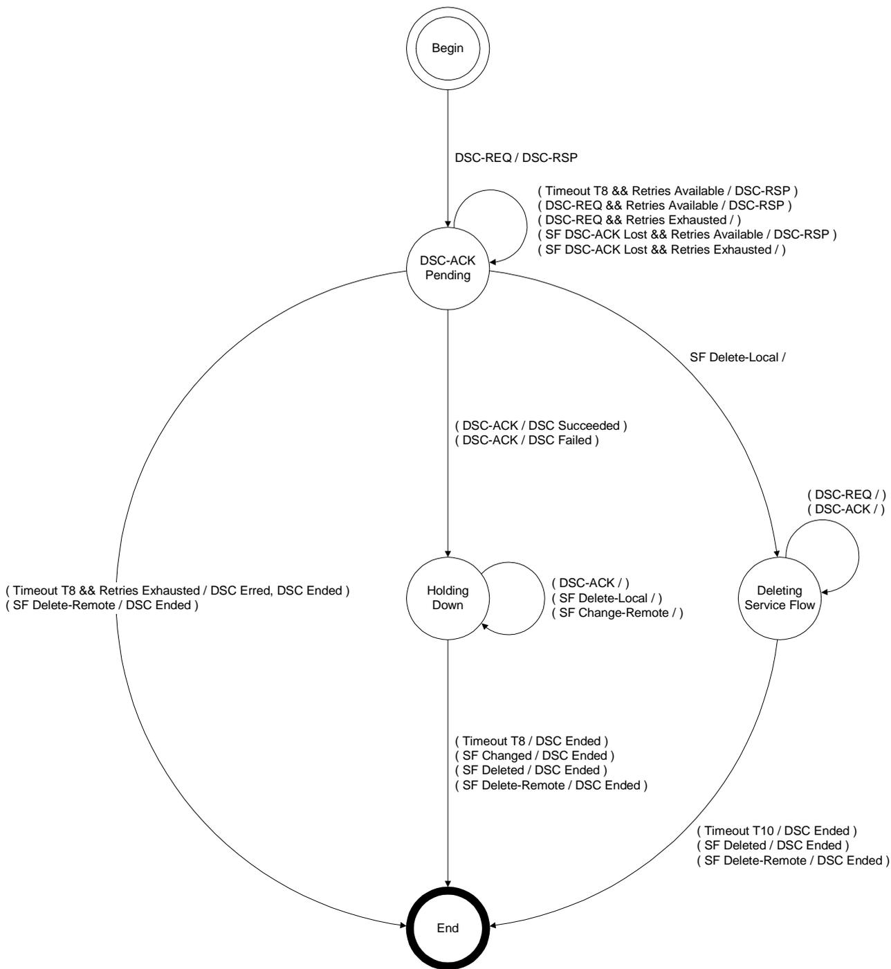
Figure 11-25: DSC-Remotely Initiated Transaction State Transition Diagram
