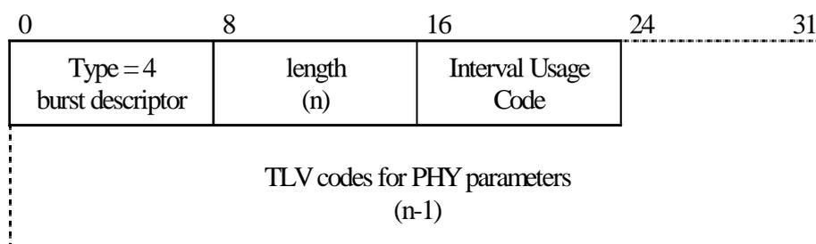
Figure 8-17: Top-Level Encoding for a Burst Descriptor
