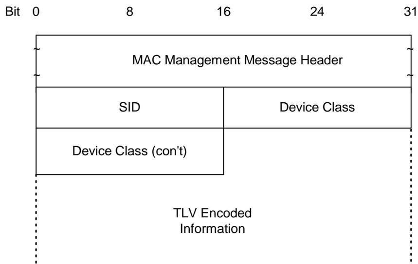
**Figure 8-42: Device Class Identification Request**
