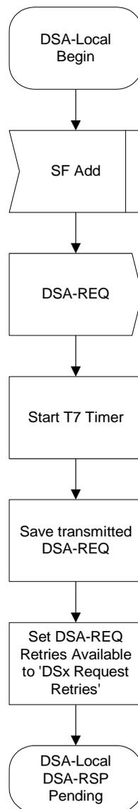
Figure 11-30: DSA-Locally Initiated Transaction Begin State Flow Diagram
