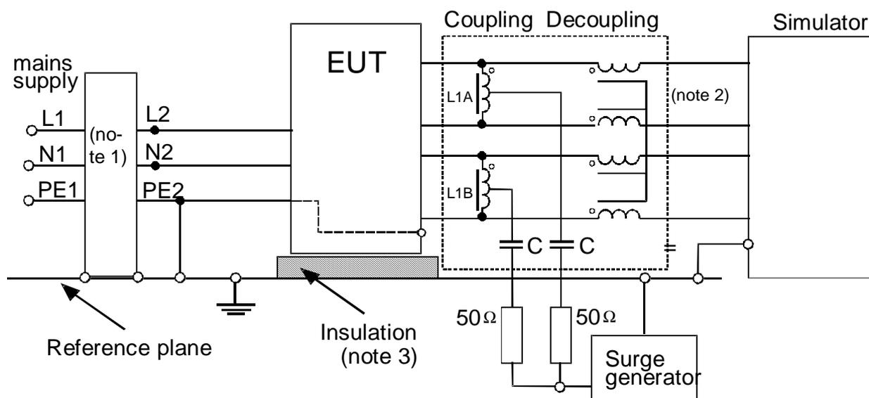
NOTE 1: The impedance matching network is used to decouple the mains and to provide low impedance to reference plane at EUT side. The impedance matching network is described in figure A.2.
