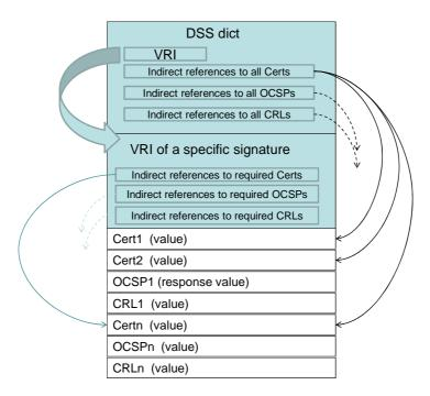
Figure 1: Illustration of DSS and VRI structures
