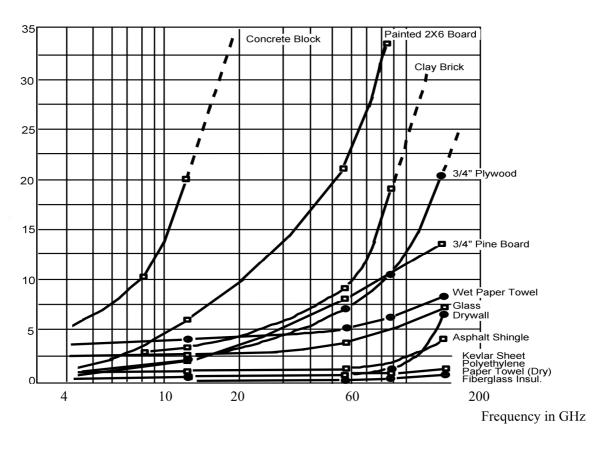
Figure C.3: Material Absorption at High Frequency in the frequency range from 3 GHz to 200 GHz in dB
