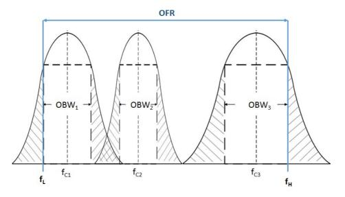
Figure 1: OFR of a multi – frequency system
