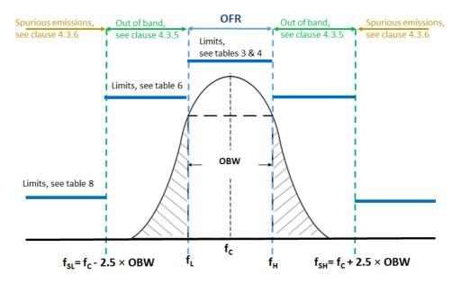
Figure 2: Emissions in the out-of-band and spurious domain
