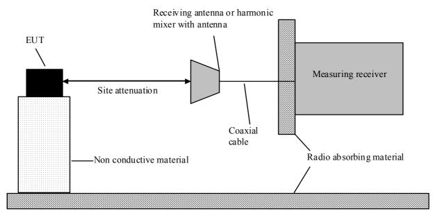
Figure 4: Example of a test site above 18 GHz with one reflecting surface
