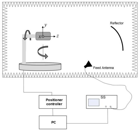
Figure B.5: IFF (CATR) measurement setup
