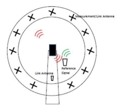
Figure B.7: Typical NFTF measurement setup
