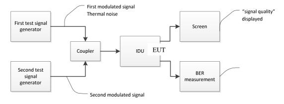
Figure 10: Test arrangement - adjacent signal selectivity
