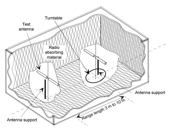
Figure B.1: A typical Anechoic Chamber
