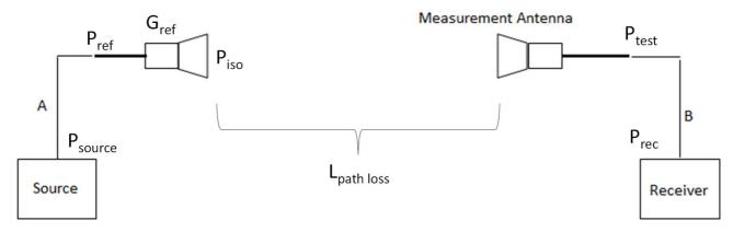
Figure B.8: NFTF - Typical setup for path loss measurement
