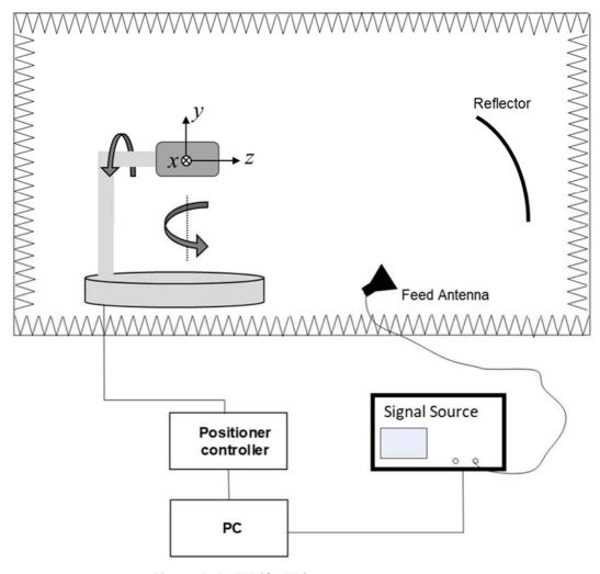
Figure B.5: IFF (CATR) measurement setup
