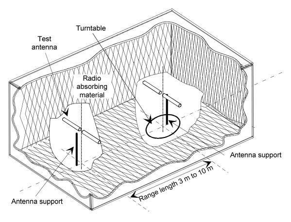
Figure B.1: A typical Anechoic Chamber
