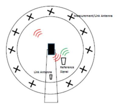
Figure B.7: Typical NFTF measurement setup
