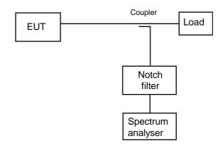
Figure 5: Test arrangement - conducted spurious radiation above the cut-off frequency
