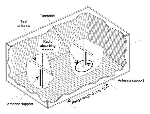
Figure C.1: A typical Anechoic Chamber
