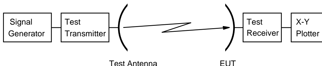
Figure 10: Test arrangement - antenna receive pattern measurement
