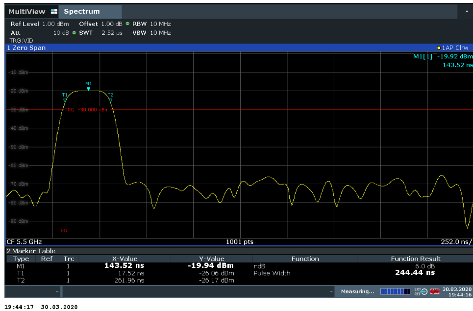
Figure F.5: Peak e.i.r.p. measurement with direct measurement where RBW > OFR
