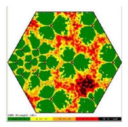
Figure 7: Typical SINR distribution of a mobile network
