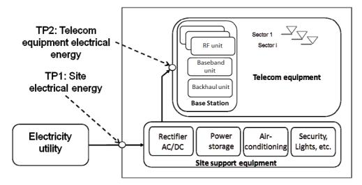
Figure 2: BS site configuration and equipment classification
