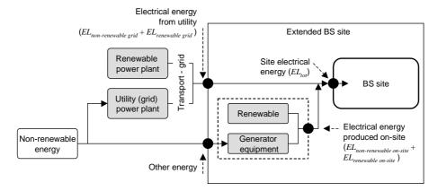
NOTE: Other energy includes chemical energy delivered to the site to generate electricity such as gasoline, etc.
