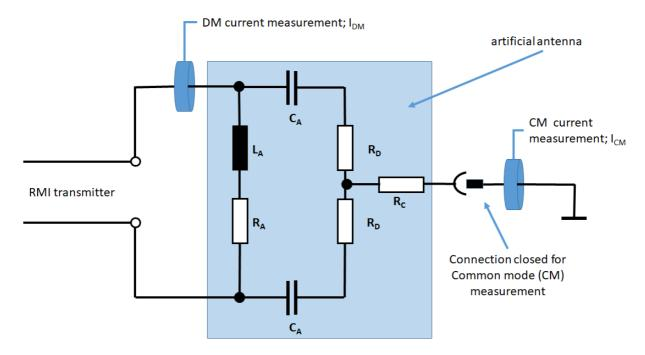
Figure B.1: Schematic of artificial antenna
