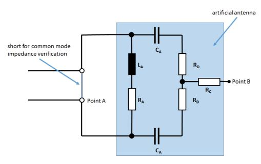
Figure B.2: Schematic for the verification of the artificial antenna common mode impedance
