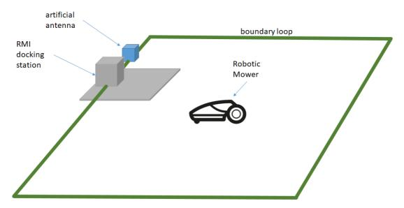
Figure 5: Schematic test set-up for RX-Sensitivity test
