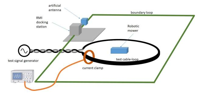
Figure 7: Schematic test set-up for the RX-blocking test 1
