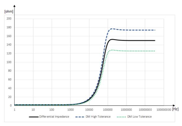
Figure B.3: Differential Mode Impedance for the RMI artificial antenna
