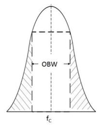
Figure 1: Occupied BandWidth (OBW)
