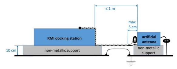
Figure B.4: Mechanical setup for measurement
