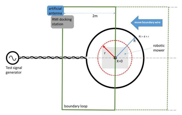
Figure 9: Schematic test set-up for the RX-blocking test 2
