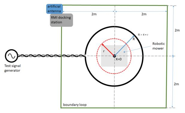
Figure 8: Schematic test set-up for the RX-blocking test 1
