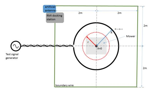
Figure 5: Schematic test set-up for the RX-blocking test 1
