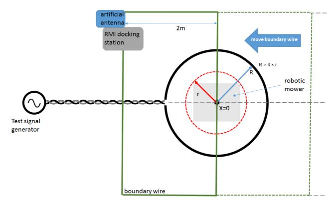
Figure 6: Schematic test set-up for the RX-blocking test 2
