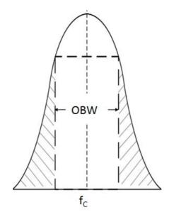
Figure 1: Occupied bandwidth (OBW)
