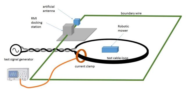
Figure 4: Schematic test set-up for the RX-blocking test 1
