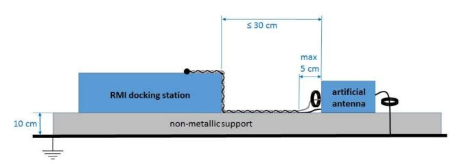
Figure C.3: Mechanical setup for artificial antenna
