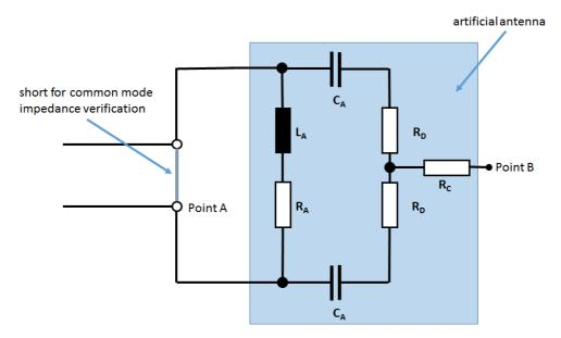
Figure C.2: Schematic for the verification of the artificial antenna common mode impedance
