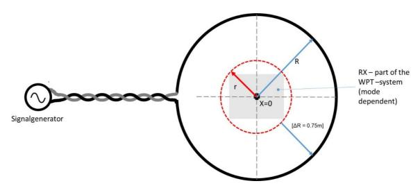
Figure 12: Schematic test set-up for the RX-blocking test
