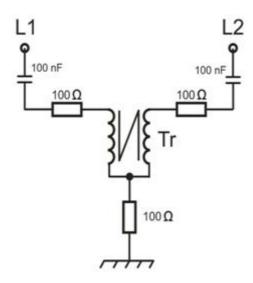
Figure 10: Example of a 150  $\Omega$  ISN
