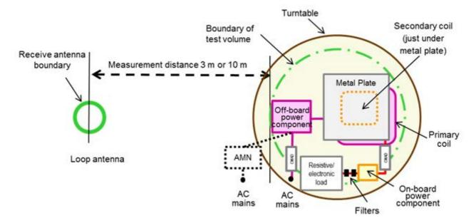
Figure B.2: Example for a typical test set up for measurement of conducted and/or radiated disturbances from a WPT equipment (primary device), Top view
