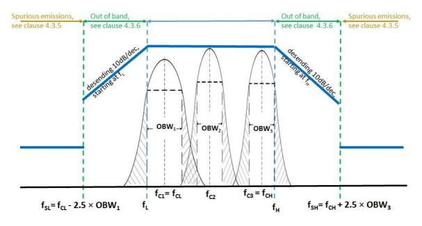
Figure 5: Out of band and spurious domain of a multi - frequency system (during one WPT system cycle time)
