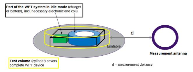
Figure 6: Setup for idle mode
