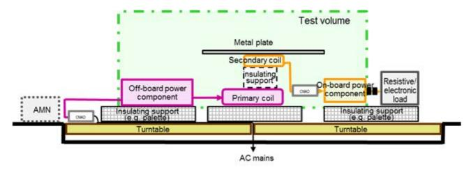
Figure B.1: Example for a typical test set up for measurement of conducted and/or radiated disturbances from a WPT equipment (primary device), Side view
