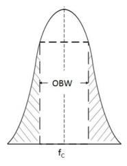
Figure 1: Occupied bandwidth (OBW)
