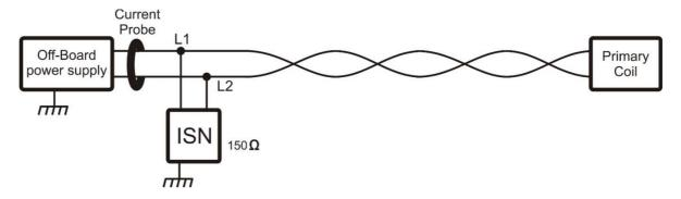
Figure 9: Measurement setup for unwanted conducted emissions
