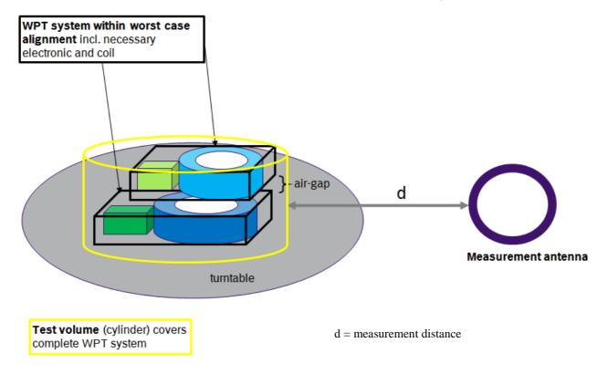
Figure 8: Setup for power transmission arrangement
