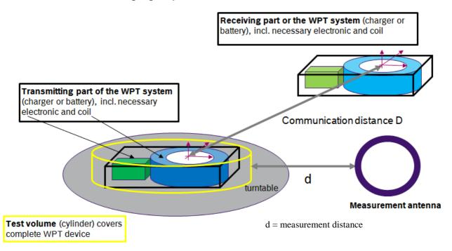
Figure 7: Setup for charging adjustment mode
