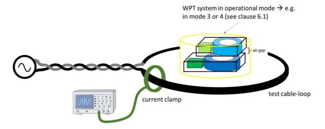
Figure 11: Schematic test set-up for the RX-blocking test
