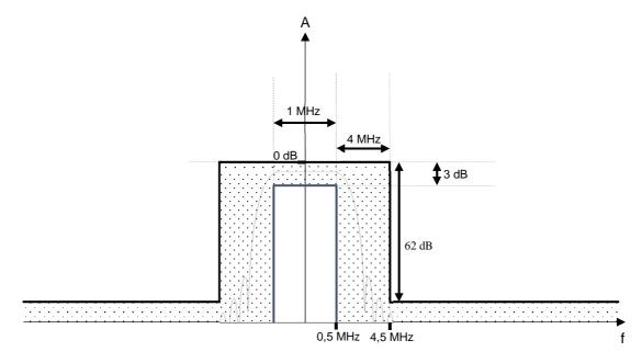
Figure B-1: Filter used to generate the blocking signal
