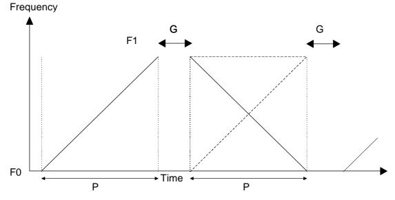
Figure E.2: Typical FMCW modulation scheme
