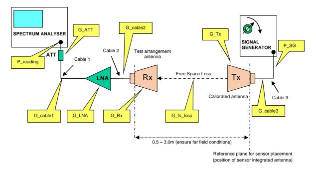
Figure C.1: Calibration set-up configuration
