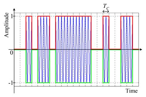
Figure E.5: Typical PN-ASK modulation scheme
