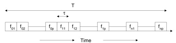
Figure E.3: Typical FSK modulation scheme
