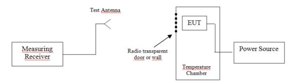
Figure A.3: Extreme conditions set-up
