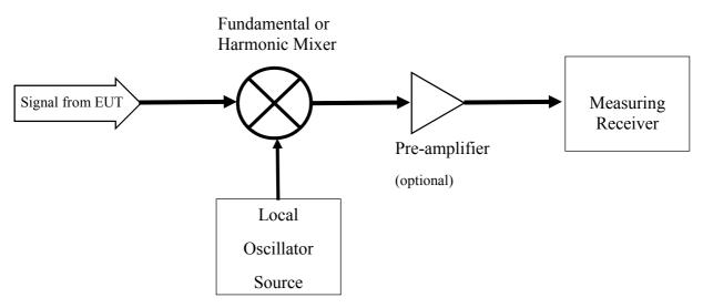
Figure D.1: Using a down-converter in front of a measuring receiver
