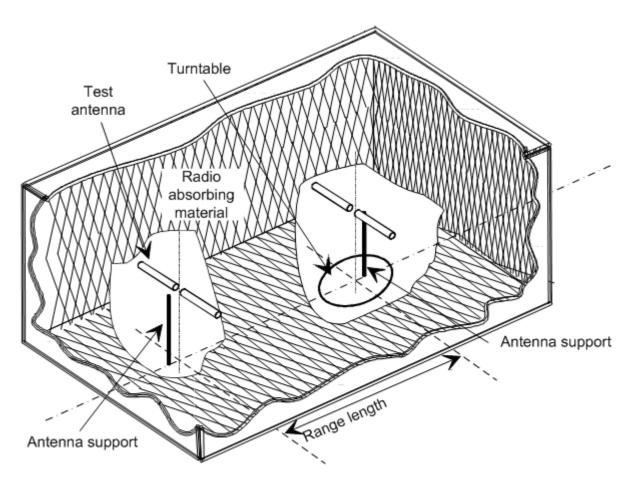
Figure A.1: A typical anechoic chamber
