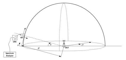
Figure 1: Azimuth and Elevation angle definitions
