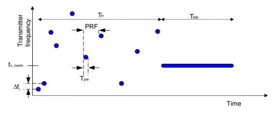
Figure E.7: Typical Pulsed FH Modulation
