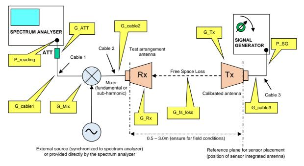
Figure C.2: Calibration set-up configuration including a mixer
