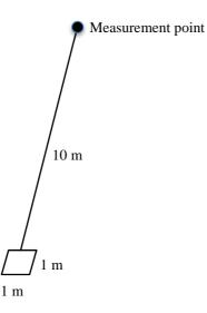
Figure B.1: 1 x 1 m loop with measurement point 10 m from the middle of one side
