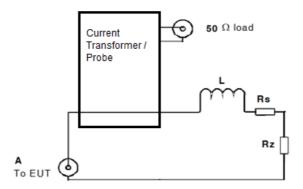
Figure D.2: Isolated test circuit
