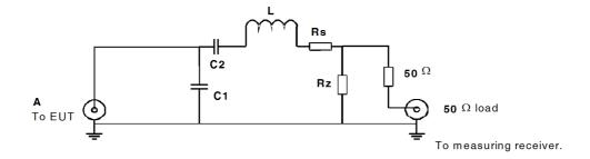
Figure D.1: Non-isolated test circuit
