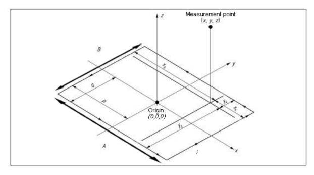
Figure C.1: Diagram for calculating magnetic field strength at point (x, y, z)
