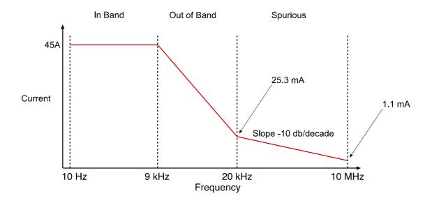
Figure E.1: Induction loop driver emissions levels and spectrum mask measurements
