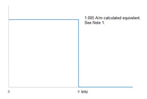
NOTE: This limit is the equivalent H-Field limit, when calculated using the formulae in clause C.1.4 of BS 7594:2011 [3], and when measured at the furthest point of the useful magnetic field volume, as declared by the provider. Actual equipment measurements are taken in terms of conducted loop output.
