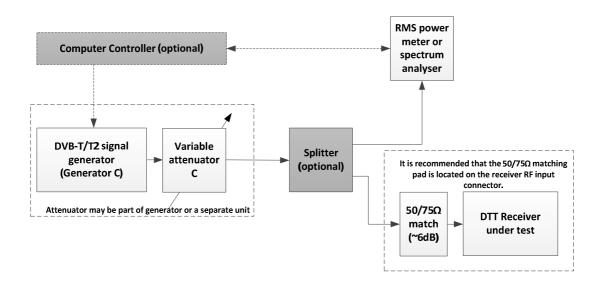
Figure 1: Measurement arrangement for sensitivity tests
