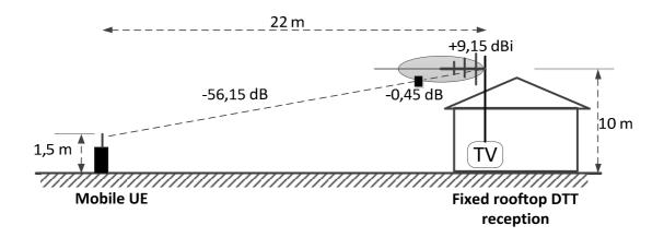
Figure B.8: Reference model for coupling gain
