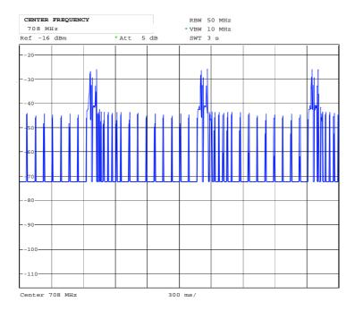
Figure B.3: Zero span plot of "short\_UE-Video-Stream\_V2" waveform (1 second loop)
